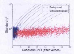
Figure 5.13: The distribution of the standard  $\chi^2$  test plotted against SNR. The majority of the background has already been removed by utilizing other signal consistency tests. The dashed lines show contours of *newSNR*, with the value of *newSNR* increasing towards the bottom right of the plot. The solid line shows the line of *newSNR* = 6; triggers above this line are discarded.
