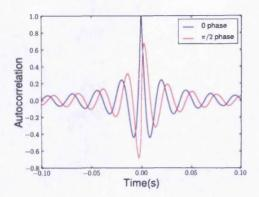
Figure 5.4: The single detector auto-correlation of a gravitational wave inspiral signal from a 1.4,1.4 solar mass binary neutron star. Both phases of the waveform are shown.
