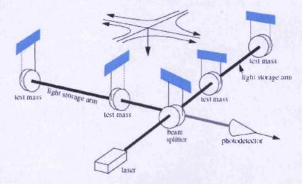
Figure 2.4: An illustration showing the principle components of a gravitational wave interferometer.
