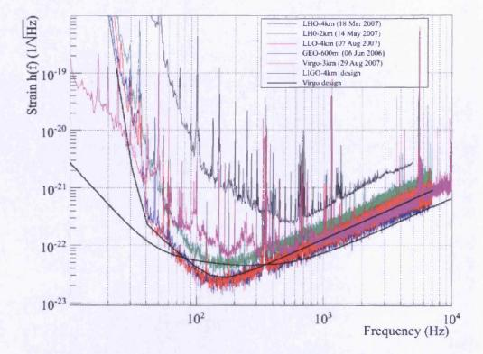
Figure 2.7: The various sensitivities of ground based detectors. The design sensitivities for the LIGO and Virgo instruments are also shown. Figure originally published in [59].
