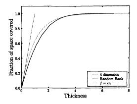
Figure 7.5: As Figure 7.3 but setting the value of  $N_{lower-bound}$  to be 50. By comparing the two figures one can see how boundary effects manifest themselves both by decreasing the initial slope df/dn and by requiring a much larger number of templates than the estimate.
