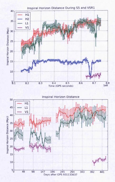
Figure 4.1: The inspiral horizon distance plotted against time for S5 and VSR1 (top) and for S6, VSR2 and VSR3 (bottom). The inspiral horizon distance is defined as the distance at which an optimally positioned, optimally oriented BNS merger would obtain an SNR of 8 in the respective detectors.
