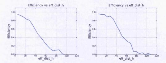
Figure 4.9: Efficiency of software injection recovery plotted against H1 effective distance for BNS injections. The left figure shows results using non-spinning injections, the right figure shows results using injections where spin is present and uniformly distributed. Injections are "found" if they are recovered with a value of effective SNR that is larger than the loudest event in the zero lag.
