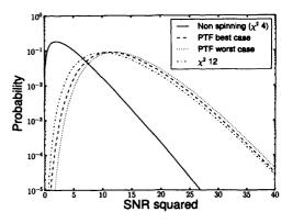
Figure 6.2: The "best" and "worst" possible distributions of the coherent PTF SNR squared as well as the distribution of the non spinning SNR squared.
