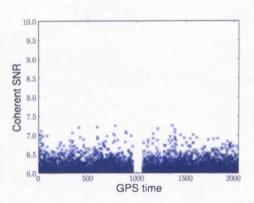
Figure 5.7: The SNR of triggers in the off-source region plotted against time for an analysis of simulated Gaussian noise in the initial LIGO (H1, H2, L1) network. The gap in the middle of the plot contains the on-source region and the buffer, this is not used in estimating noise background rates. The loudest trigger occurs with an SNR of 7.24.
