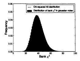
Figure 5.3: The distribution of the bank  $\chi^2$  test for a single template h, with a bank of size 10. The plot shows the distribution of the bank veto calculated for every time sample in 128s of simulated Gaussian data (with no signal present). In the case that the ten bank templates are orthogonal, the expected distribution is  $\chi^2$  with 40 degrees of freedom (shown as the solid black line). As can be seen, the actual distribution follows the expected one closely.
