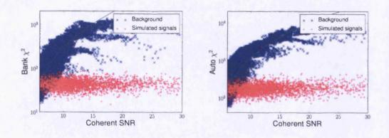
Figure 5.12: The distribution of bank and auto  $\chi^2$  test plotted against SNR. There is a clear separation between simulated signal and background at coherent SNRs above 10. The solid line shows the line of newSNR = 6. Triggers with newSNR < 6 (above and to the left of the line) are discarded.
