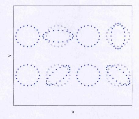
Figure 2.1: The deformation of a ring of particles due to the passage of a + polarized gravitational wave (top) and a × polarized wave (bottom), propagating in the z direction. From left to right we show the  $0, \frac{\pi}{2}, \pi$  and  $\frac{3\pi}{2}$  phases. The unfilled circles denote the positions of the particles at the 0 phase. This Figure was originally published in [38].
