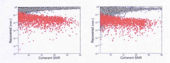
Figure 5.1: The distribution of the recovered inclination angle plotted against coherent SNR for optimally oriented signals (unfilled circles), uniformly distributed orientations (blue crosses) and simulated glitches (red circles). The left figure shows a network configuration where we are equally sensitive to both gravitational wave polarizations. The right figure shows a configuration where we are 5 times more sensitive to the + polarization than to the  $\times$ .
