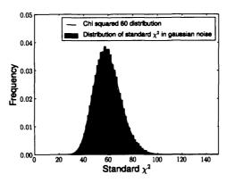
Figure 5.6: The distribution of the standard  $\chi^2$  test for a single template h, split into 16 non-overlapping frequency bins. The plot shows the distribution of the  $\chi^2$ test calculated for every time sample in 128s of simulated Gaussian data (with no signal present). The observed distribution of values (shown in grey) is an excellent match with the expected  $\chi^2$  distribution with sixty degrees of freedom (shown in black).
