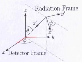
Figure 2.5: An illustration of the angles that describe the relationship between the detector and radiation frames. Figure originally published in [38].
