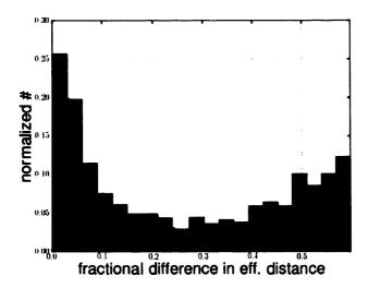
Figure 4.6: A histogram of the fractional difference in effective distance. The distributions for simulated signals (red) and background triggers (black) are shown. Here triggers with a fractional difference bigger than 0.6 have been removed.
