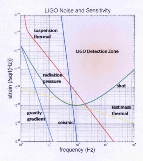
Figure 2.6: An illustration of the sensitivity of current gravitational wave interferometers, highlighting how different noise sources will determine the strain sensitivity of the instrument. Figure originally published in [58].
