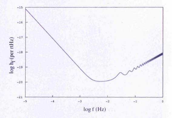
Figure 2.8: A diagram showing the predicted sensitivity curve of the proposed space-based LISA detector. Figure originally published in [63].
