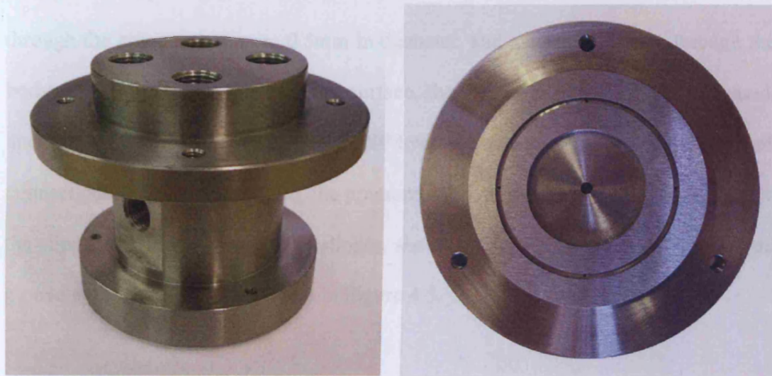
Figure 4.4 a: Slipper with hydraulic connections b: Slipper face
