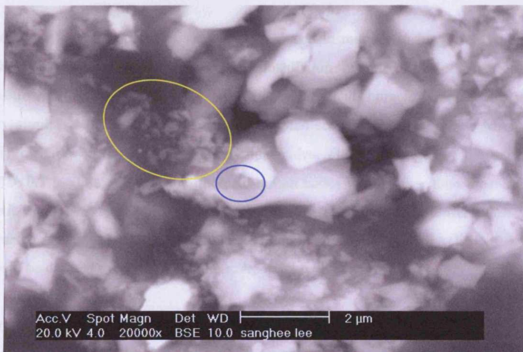
Figure 5. 25 The BSE images of the MA remaining in the lung at 49 weeks post-exposure. Blue circles depict the particles attached to a larger one. Yellow circle depict the particles, which are not attached to any other particles.
