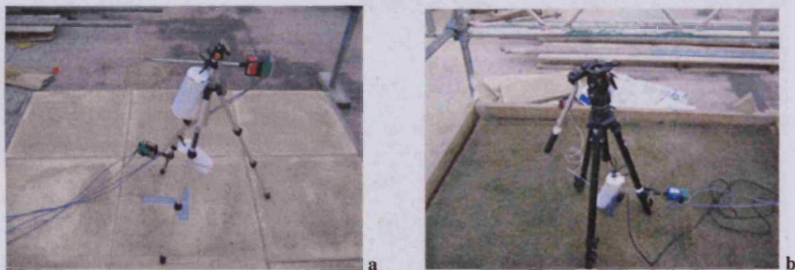
Figure 158. Partial view of (a) concrete and (b) green test cell with their sensors
