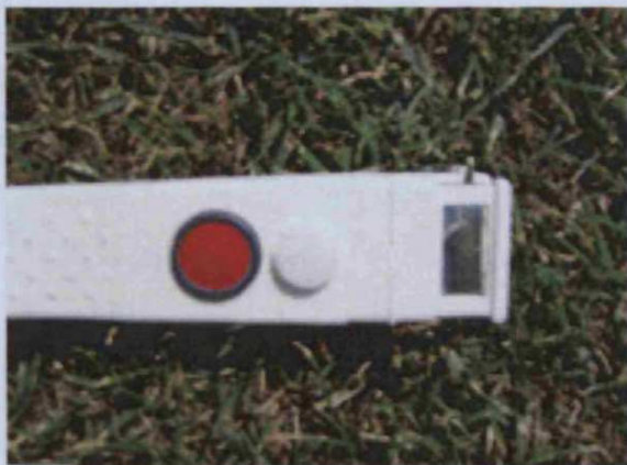
Figure 175. The head unit of the \Delta T AP4 Porometer, measuring a leaf stomatal resistance during the experiment
