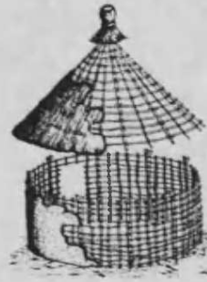
Figure 71. Structural sketch of the redondo house, in Cuajuinuilapa, Mexico (Oliver, 1997c)
