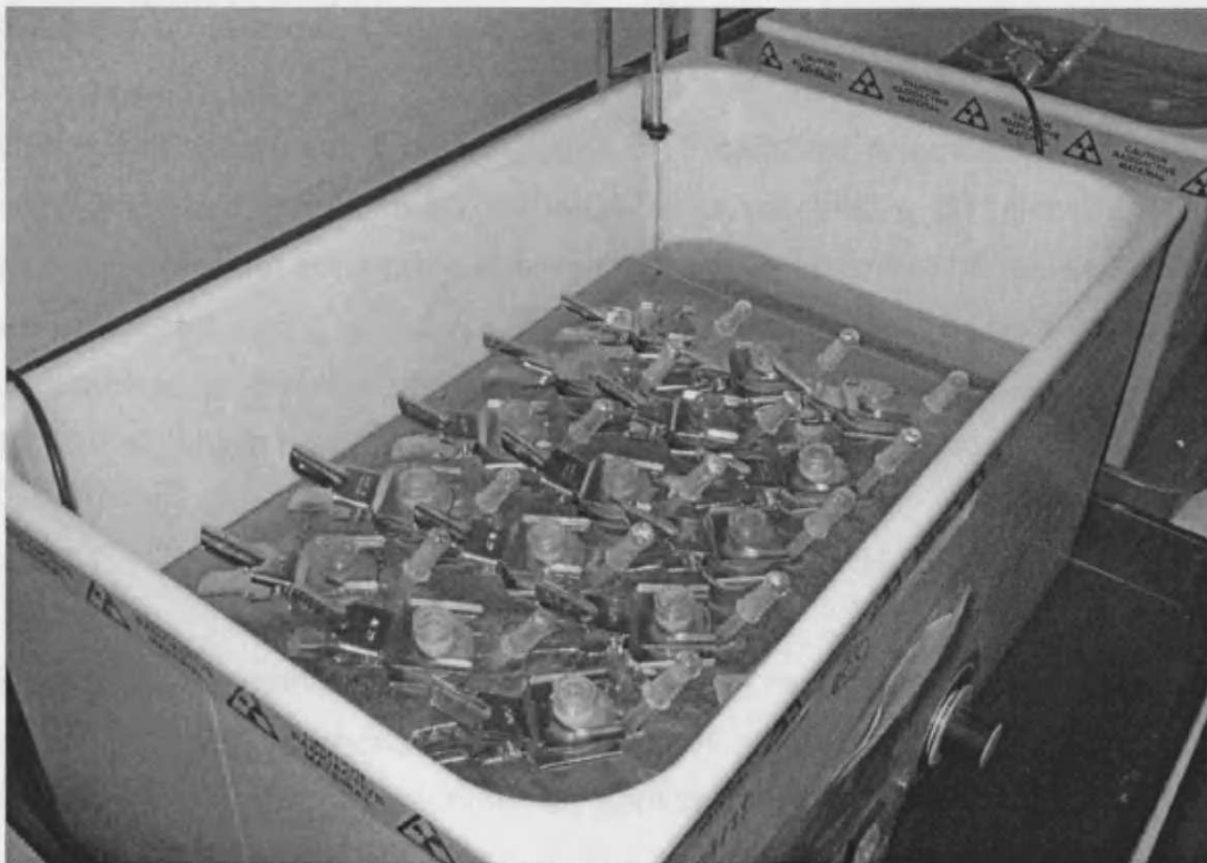
Figure 4.2 The experimental diffusion cell set-up
