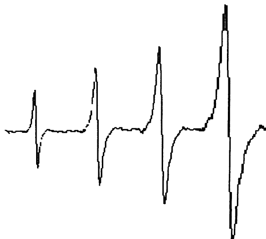
Figure 30 Schematic representation of the effect of rotational correlation time on copper(II) spectrum
