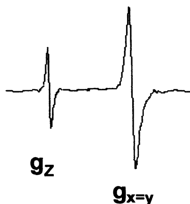
Figure 32 Schematic of spectrum obtained from fully hydrated copper ion experiencing a Jahn-Teller distortion
