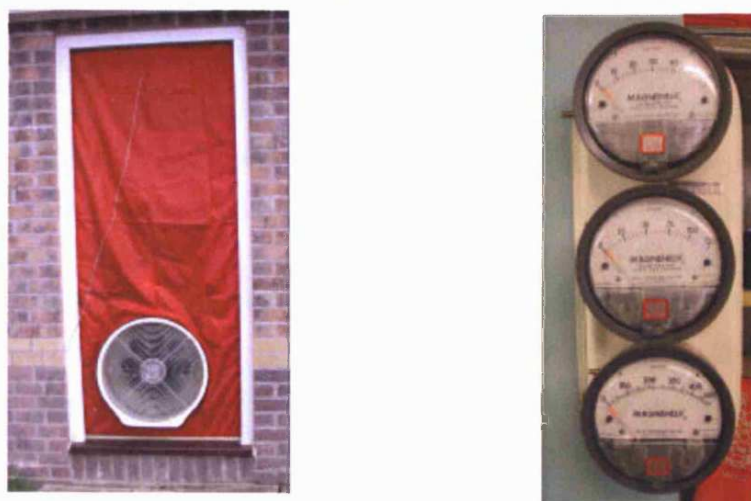
Figure 99: Typical Fan Pressurisation Equipment for Domestic Scale Air Leakage Tests
