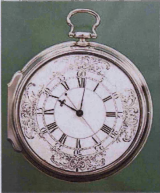
Fig 2.117 John Harrison's H4 Chronometer.
