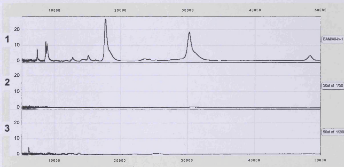
Figure 3.8 Spectra of three spots on a Q10 ProteinChip array in a sample volume optimisation experiment using different dilutions.
