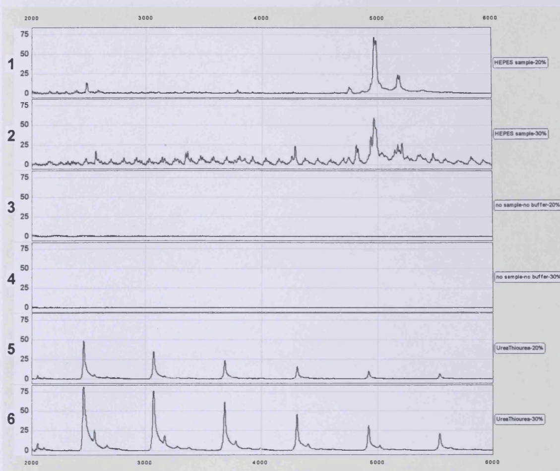
Figure 3.19 Spectra of six spots testing if the urea-thiourea lysis buffer was causing the signal repeat. The spectra correspond to three fractionations on an NP20 ProteinChip: 1-2 20% and 30% fraction of 50 \mu l homogenate of half cerebra of 10 week old transgenic R6/1 in HEPES lysis buffer in a total volume of 200 \mu l of 10% ACN and 0.5% TFA; 3-4 20% and 30% fraction of 200 \mu l of 10% ACN and 0.5% TFA without sample; 5-6 20% and 30% fraction of 50 \mu l urea-thiourea lysis buffer without protein in a total volume of 200 \mu l of 10% ACN and 0.5% TFA. Only spectra 5 and 6 show the signal repeat.
