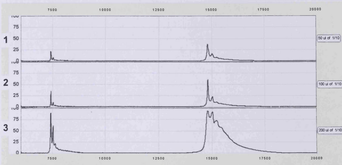
Figure 3.10 Spectra of three spots on a Q10 ProteinChip array in a sample volume optimisation experiment using the same dilution in different total volumes. A 1/10 dilution of Chicken Lysozyme in different volumes of 50 mM CAPS buffer was applied:
