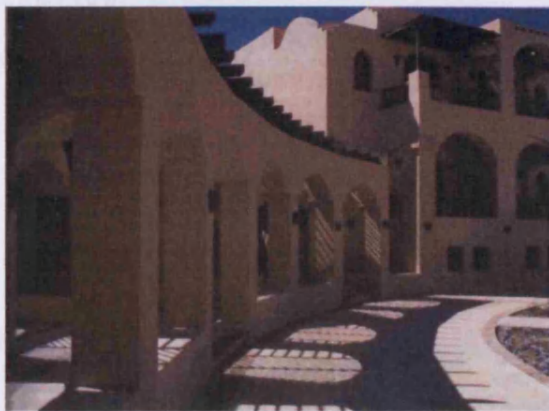
Figure 3- 19: The façade composition to maximize shades. (Source: Albenaa, 1999)
