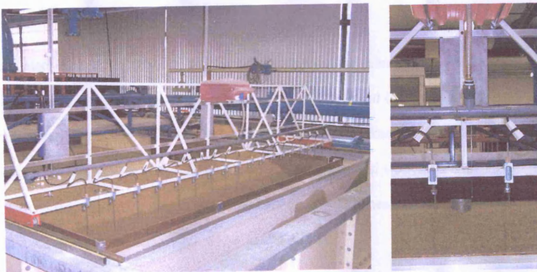
Figure 5.23: General view of dye tracer device and nozzles
