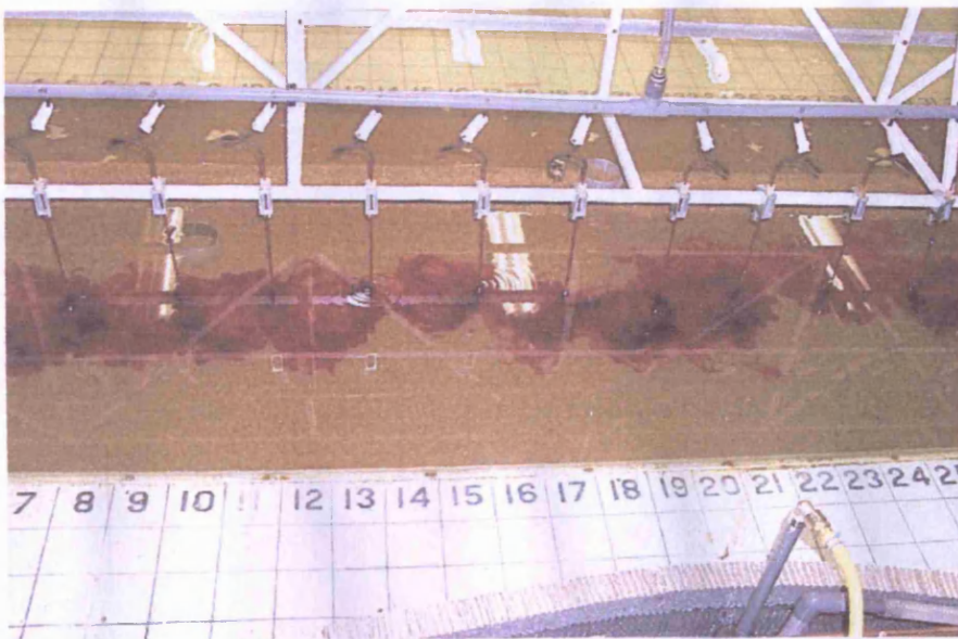
Figure 5.27: Release of dye tracer along a line
