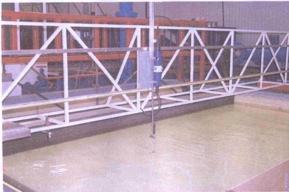
Figure 5.20: ADV down-looking probe during operation
