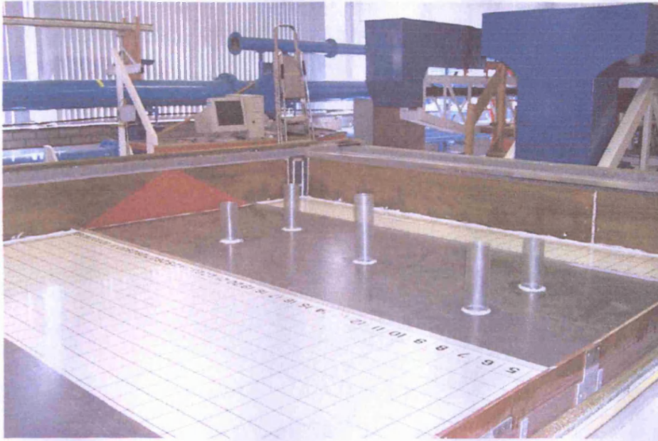
Figure 5.15: Physical model observation wells
