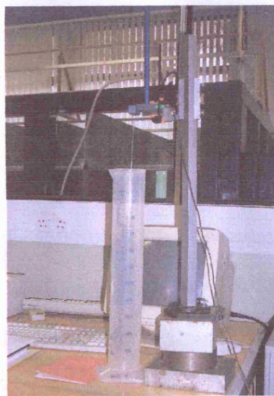
Figure 5.19: Calibration of wave probe monitor
