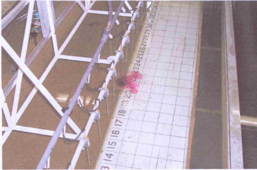
Figure 5.26: Release of dye tracer at a point
