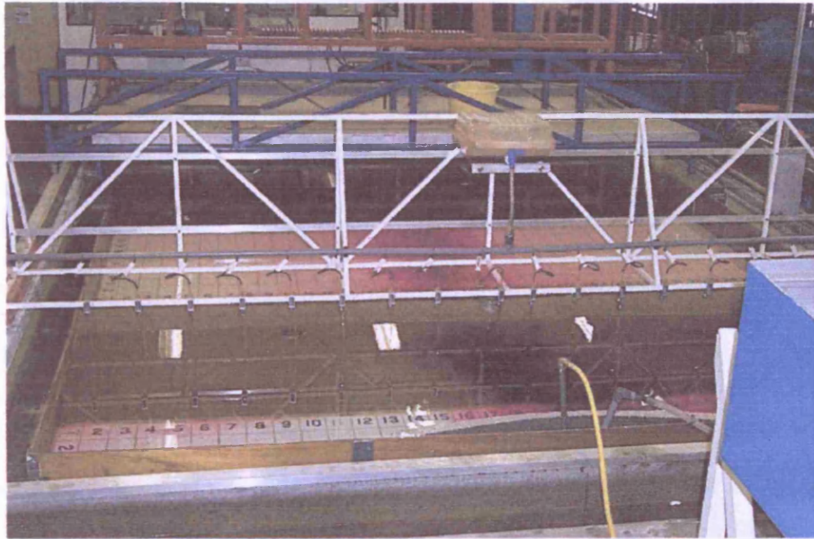
Figure 5.28: Overall condition of dye tracer experiment after 30 min., single point test
