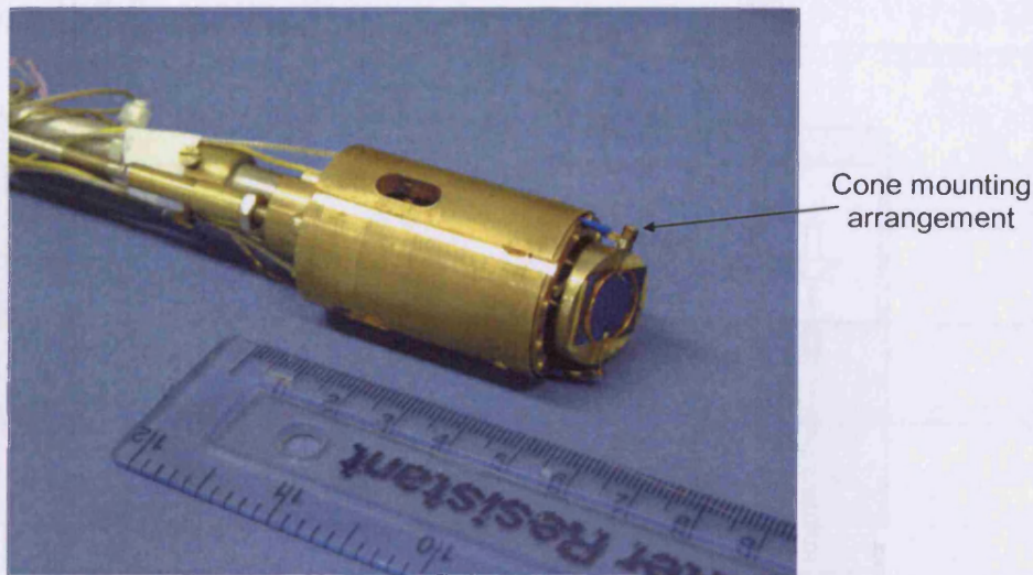
Figure 4.6: Photograph of Mark IIIb, showing the GaAs rotor fitted with calibration coil, the cone and drawbar mountings and the fibre supports (stator plates concealed behind the rotor).
