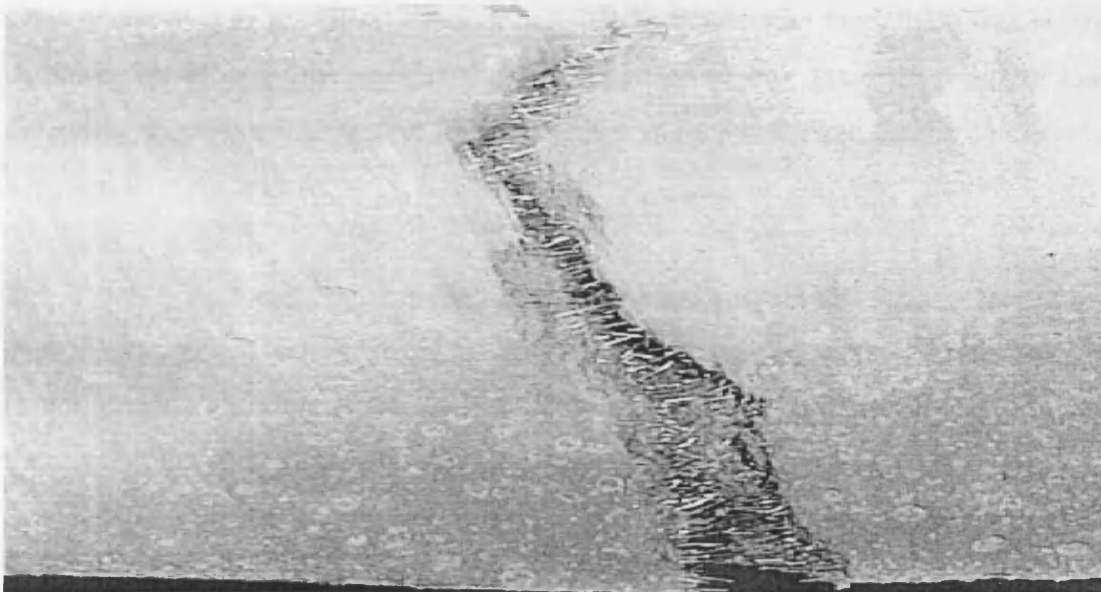
Plate 7.9 Bridging action of steel fibres.
