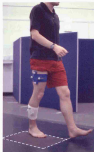
Figure 2.8 A walking trial showing the subject walking along the raised walkway and cleanly contacting the force platform (highlighted by the dotted white line) in the stance phase.
