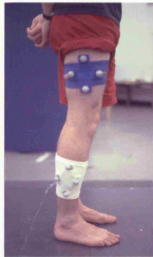
Figure 2.5 The marker clusters are positioned laterally on the shank and thigh and are held in position using self-adhesive tape or tubigrip.
