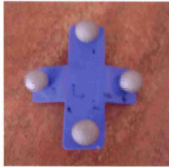
Figure 2.4 A rigid marker cluster covered with four retro-reflective markers.
