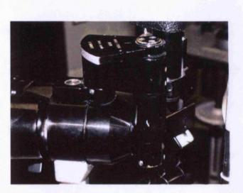
Fig 3.5: The Haag-Streit Pachometer attached to a slit-lamp for the measurement of corneal thickness.
