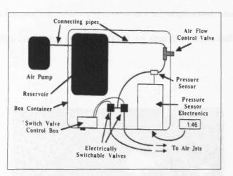
**Figure 3.1:** Diagram of the technical components of the Non Contact Corneal Aesthesiometer (NCCA) (From Murphy PJ et al: Ophthal Physiol Opt 16: 101-107, 1996).
