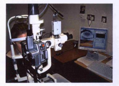
Fig 2.10: Camera set-up for the measurement of the ocular surface temperature.
