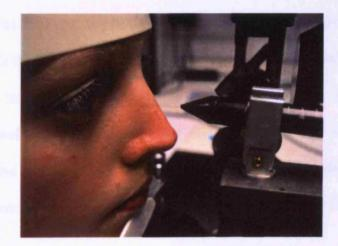
Fig 3.4: Nylon monofilament of the Cochet-Bonnet aesthesiometer moving towards to the eye.
