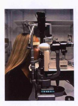
**Picture 3.6:** Set-up of the Tearscope for the measurement of the tear-film break-up time non-invasively.
