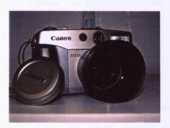
**Fig 3.14:** Digital Canon Camera Power Shot G2, attached to a close-up lens Canon (250D, 58mm), through a conversion lens adapter.
