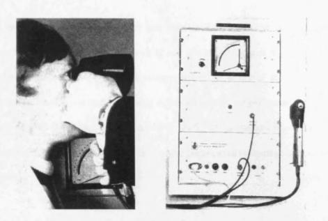
Fig 2.12: Mastpone's bolometer set-up (Mastpone, 1968b).
