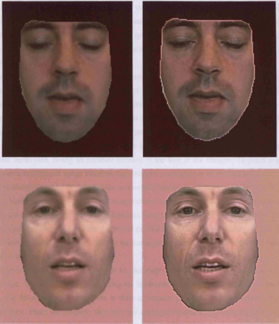
Figure 9.4: Unsharp masking to improve facial detail. The image produced by hierarchical model 2 (top right) appears slightly distorted after unsharp masking. This processing step is therefore not applied to hierarchical model 2 animations. The image produced by hierarchical model 1 (bottom right) is greatly enhanced by unsharp masking. This process is therefore applied by default to all hierarchical model 1 animations. The decision to apply unsharp masking is therefore based solely on ascetic considerations.
