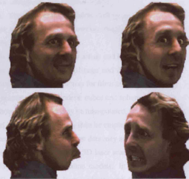
Figure 2.4: Animation of a muscle based model generated automatically from laser-scanned range and reflectance data. The model may subsequently be animated by relaxing and contracting the muscles in the model [96].
