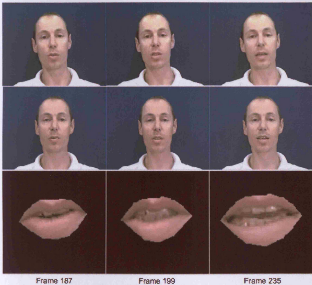
Figure 11.22: Selected frames from the synthesised sentence “And tried a mouthful of the next bowl of porridge. Too sour she said.”. Synthesis is achieved using a mouth HMCM constructed with hierarchical model 2.
