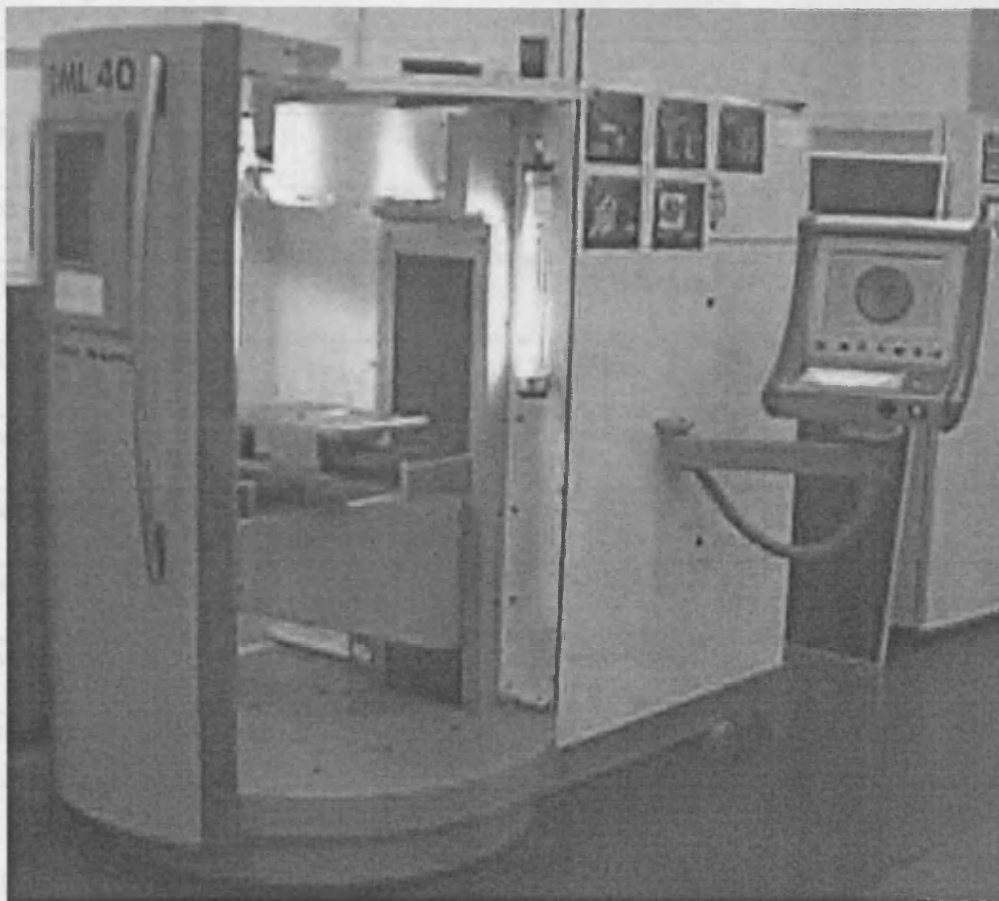
Figure A.1 The DML 40 SI laser milling machine
