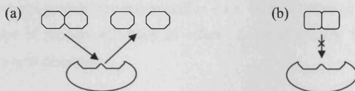
Figure 1.8: (a) Successful interaction and subsequent dissociation of a molecule on an active site and (b) no reaction occurring between an active site and a species of the wrong shape.
