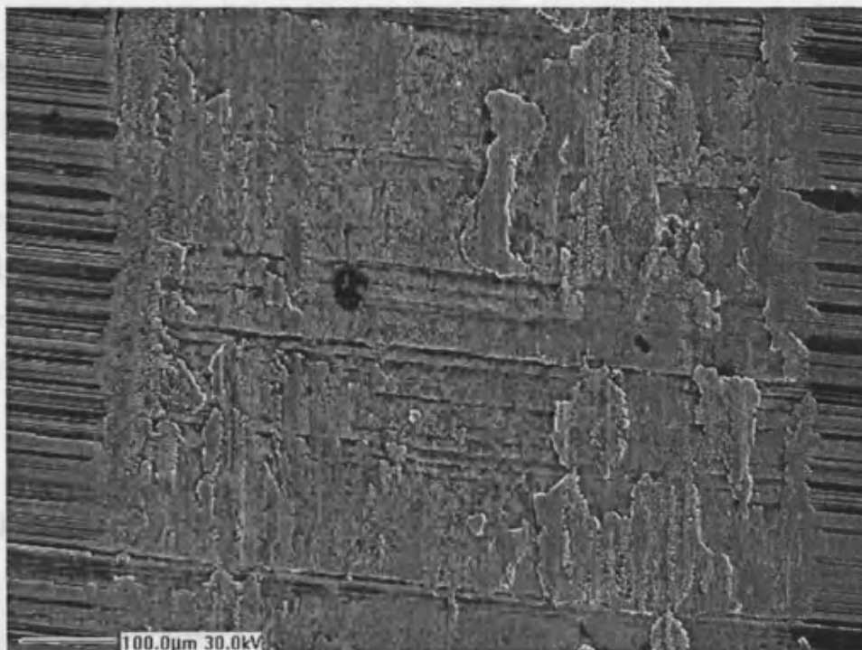
Figure 1.3 – SEM image of the scuffed region of a test disk
