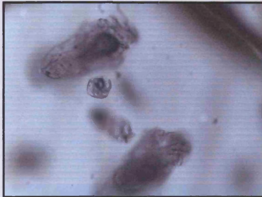
Fig. 4.5. Several inclusions hosted in olivine, the larger inclusions have elongated to irregular shapes being \sim 30 \mu\text{m} in length and 5\text{-}15 \mu\text{m} in width. The sample is from the Mull Plateau Group lavas; sample BM2, Grid Reference [NM 874784], altitude 157m.
