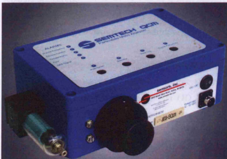
Figure 3.1: A Quartz Crystal Microbalance (QCM) Mass Monitor produced by Sensors Inc. under the licence of Booker Systems Ltd. (Source: www.news.thomasnet.com )
