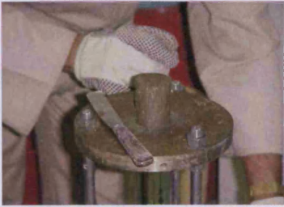
Plate 5.3. Extracting and levelling the soil specimen
