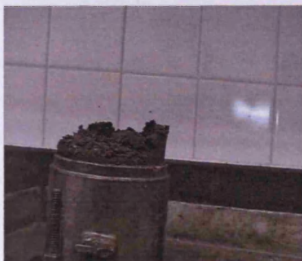
Plate 4.3. Expanded soil samples during compaction
