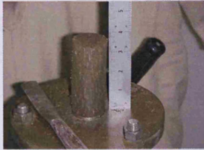
Plate 5.3. Extracting and levelling the soil specimen
