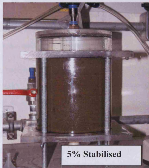
Plate 7.3. Natural and stabilised Sabkha soils after leaching with 20 pore volumes
