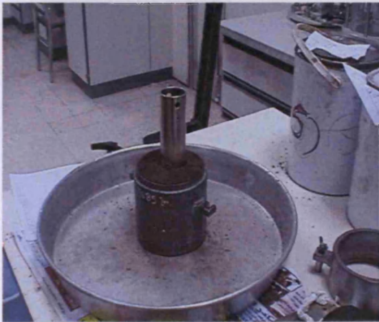
Plate 5.2. Removing the tube containing the soil from the mould
