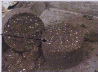
Plate 7.2. Partially coated salts in 5% stabilised Sabkha soil samples
