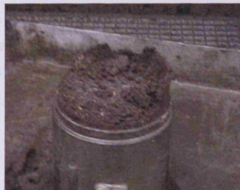
Plate 4.3. Expanded soil samples during compaction
