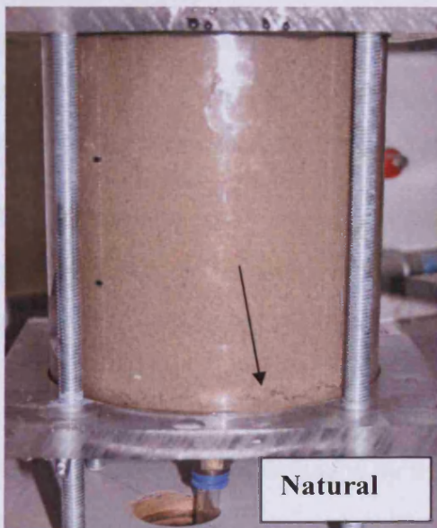
Plate 7.3. Natural and stabilised Sabkha soils after leaching with 20 pore volumes
