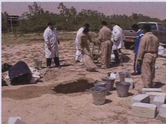
Plate 8.2. Mixing the Sabkha soil with oil residue
