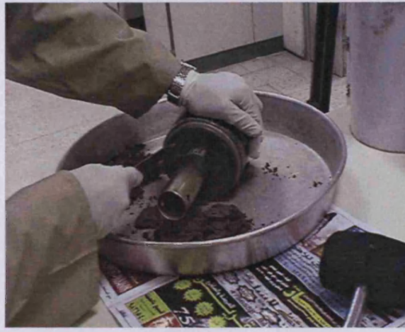
Plate 5.2. Removing the tube containing the soil from the mould
