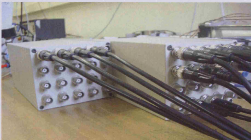
Figure 3.22: DAP I/O channel interface
