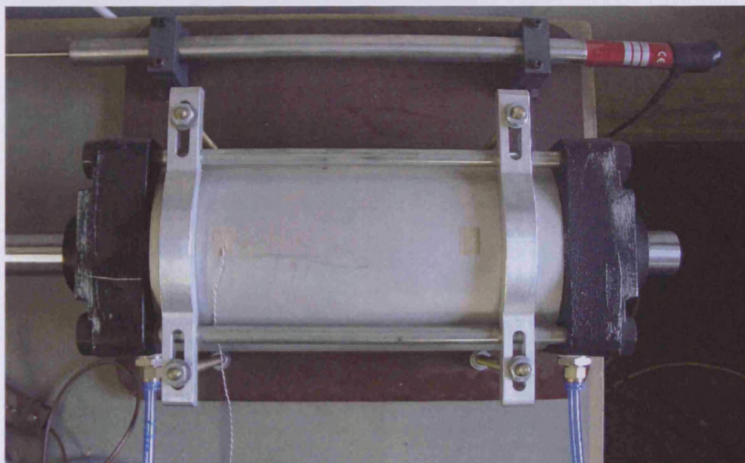
Figure 3.12: LVDT ACT 3000C mounted at the side of the pneumatic cylinder
