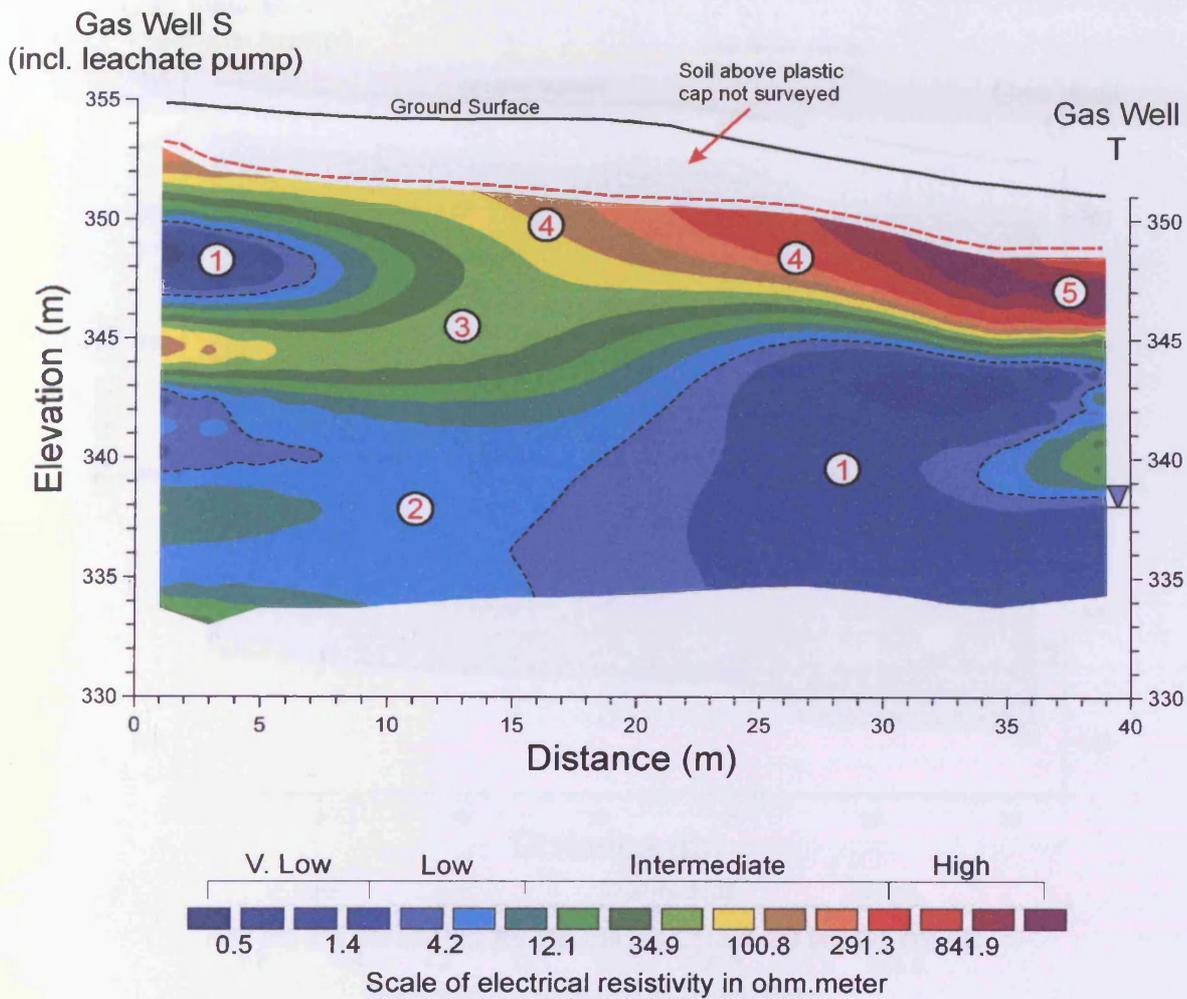
Figure 6.15: ERT results between gas wells S to T recorded during February 2006 after one month of leachate pumping.
