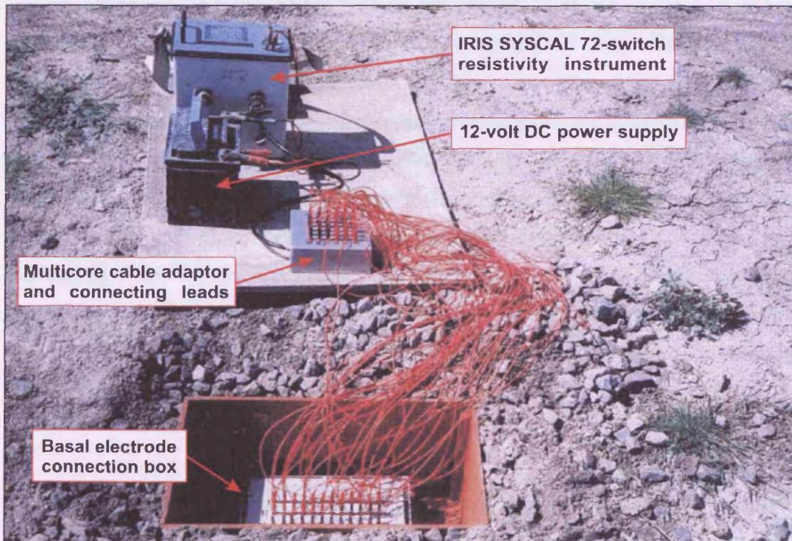
Figure 5.10: A photograph illustrating connection of the concealed basal electrodes to the resistivity acquisition instrument at the control box location (author).
