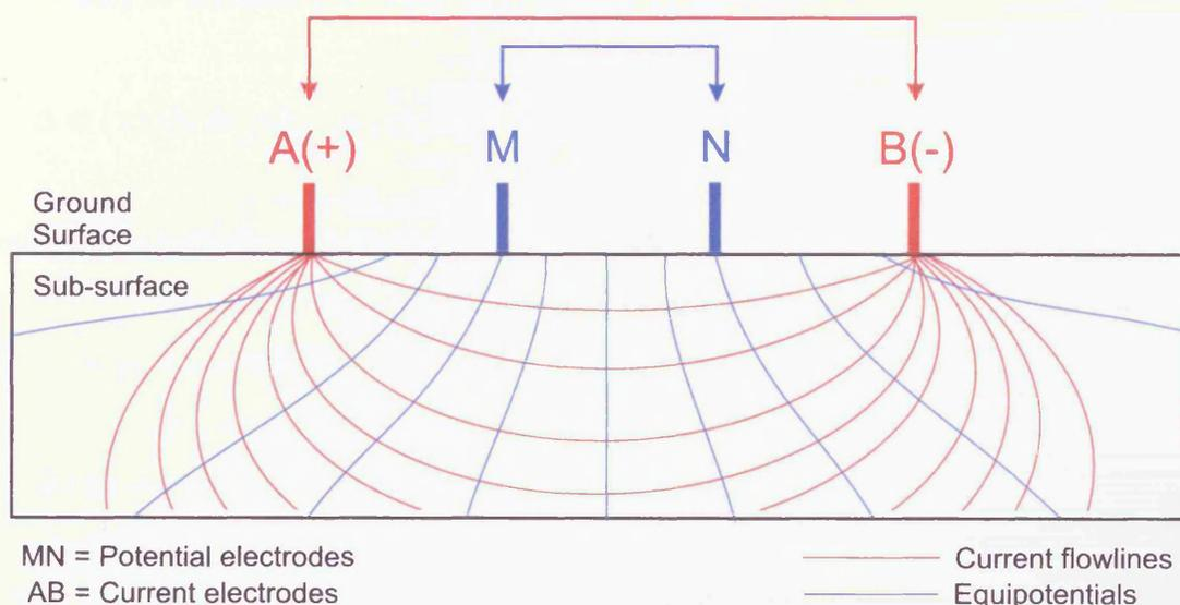
Figure 2.1: A diagram illustrating the basic theory of ground resistivity measurement by introducing electrical current and measuring voltage potential.
