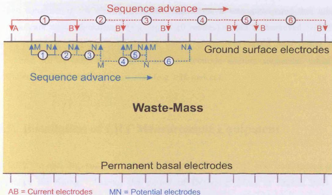
Figure 5.3: *Electrode address sequence for ABMN along the ground surface array only, showing a sample set of measurements.*
