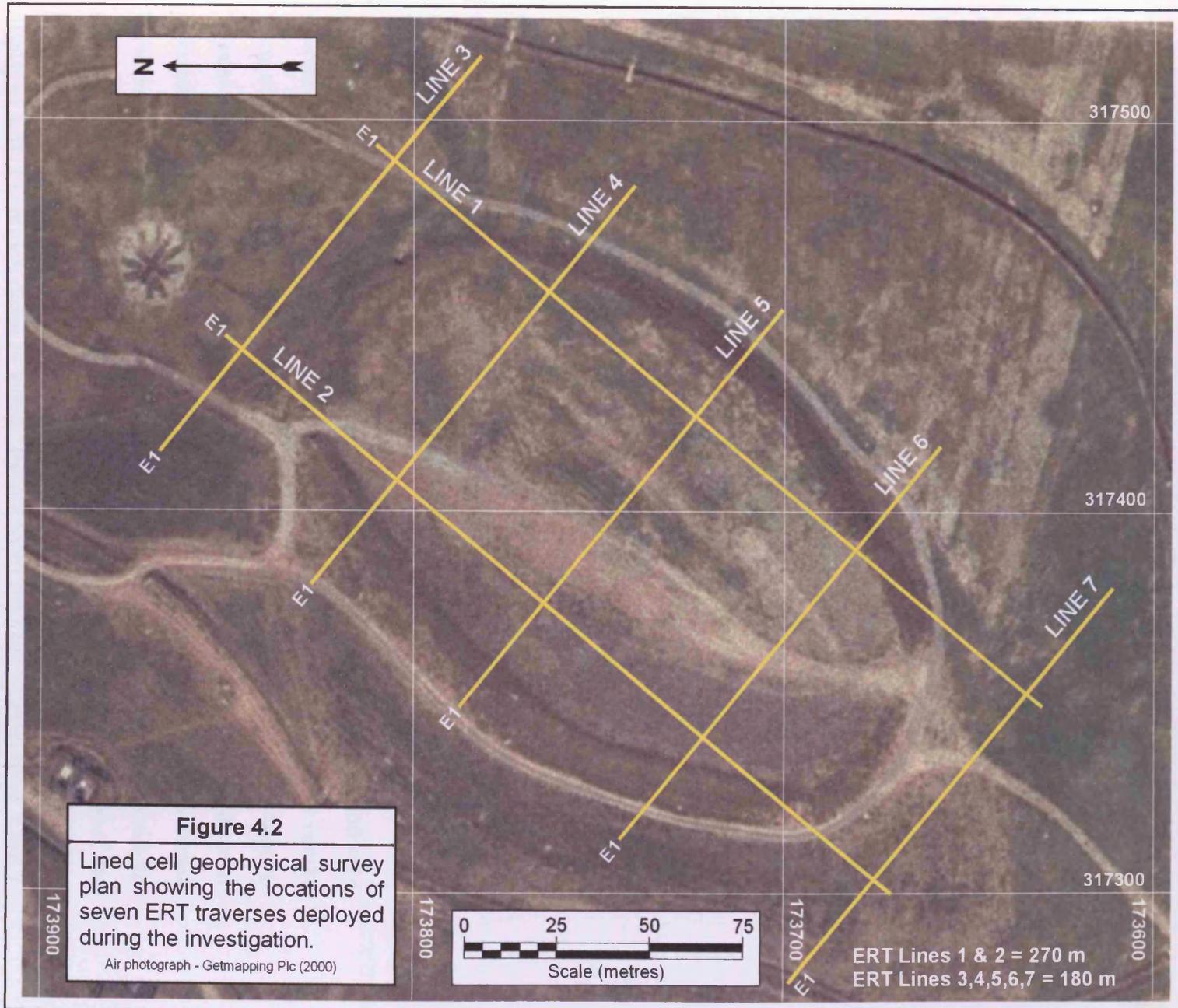
In order to provide a comparison with ground conditions outside the margins of the disposal cell, lines 3 and 7 were positioned beyond the perceived extent of the HDPE liner, as documented in Figure 3.8 of the desk study.
