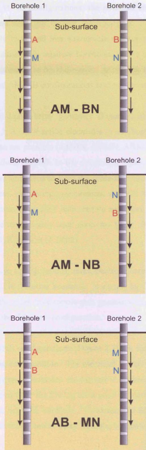
Figure 2.5: A diagrammatic representation of the three electrode configurations of the cross-hole dipole-dipole borehole ERT array geometry (after Goes and Meekes, 2004).
