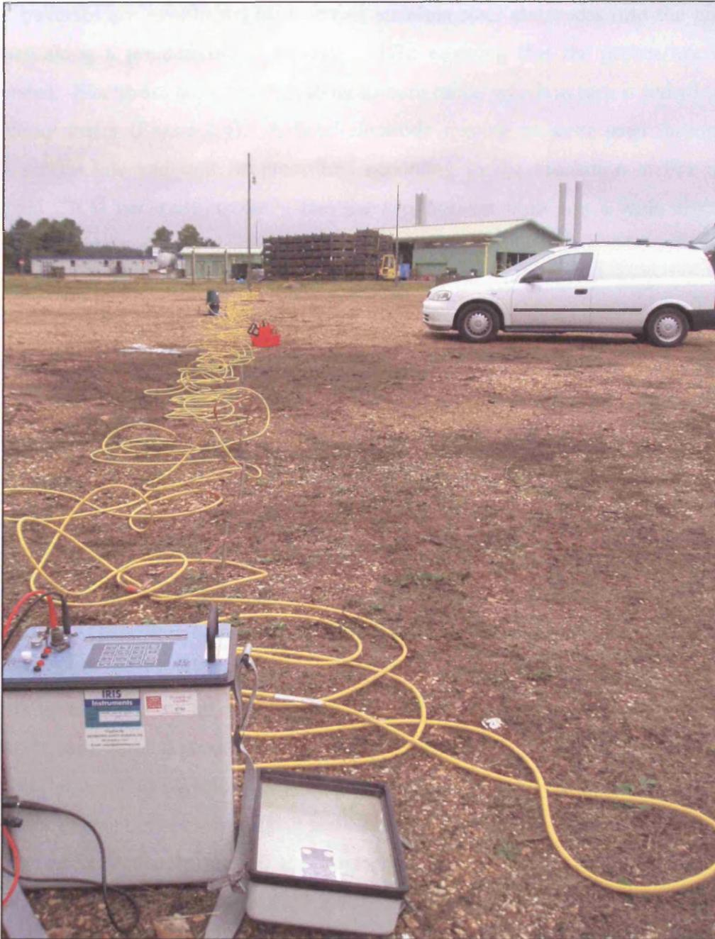
Figure 2.4: *A photograph illustrating ERT data acquisition during a geophysical site characterisation (author).*
