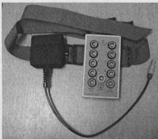
Figure 2.19: Patient unit with waist belt and battery pack.
