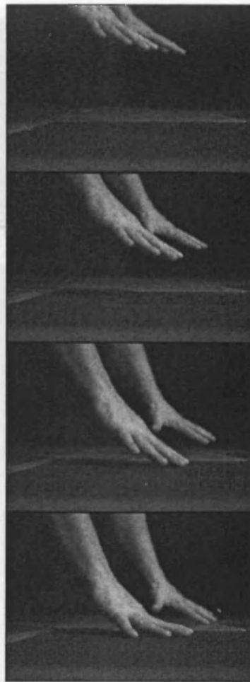
Figure 3.49: Series of still photographs taken from high-speed video footage, showing a fall onto the force plates from kneeling height (male volunteer).
