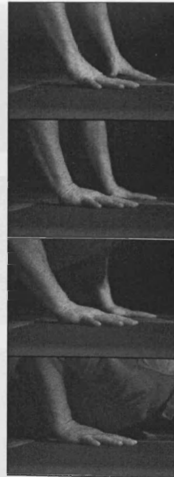
Figure 3.49: Series of still photographs taken from high-speed video footage, showing a fall onto the force plates from kneeling height (male volunteer).
