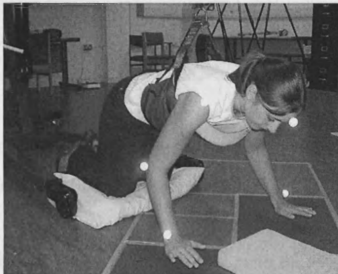
Figure 2.12: Volunteer suspended in harness from drop rig with each hand positioned over the force plates.
