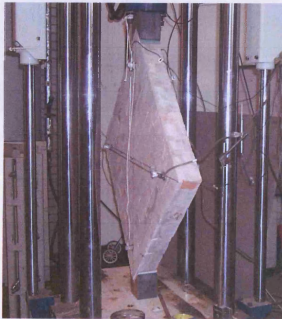
Plate 4.12- Set up for the prototype diagonal tensile strength test.
