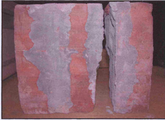
Plate 5.4- Shear failure in prototype specimens.
