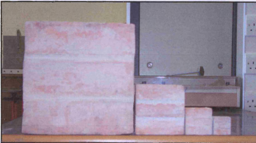
Plate 4.3- Triplet specimens in the four scales.
