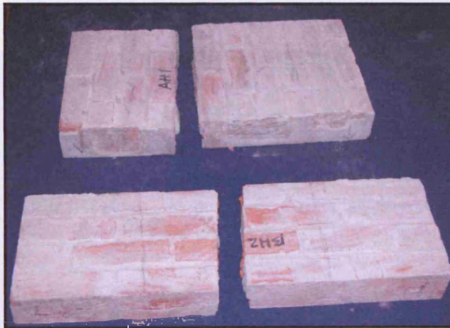
Plate 5.5- Failure in half scale flexural strength specimens.
