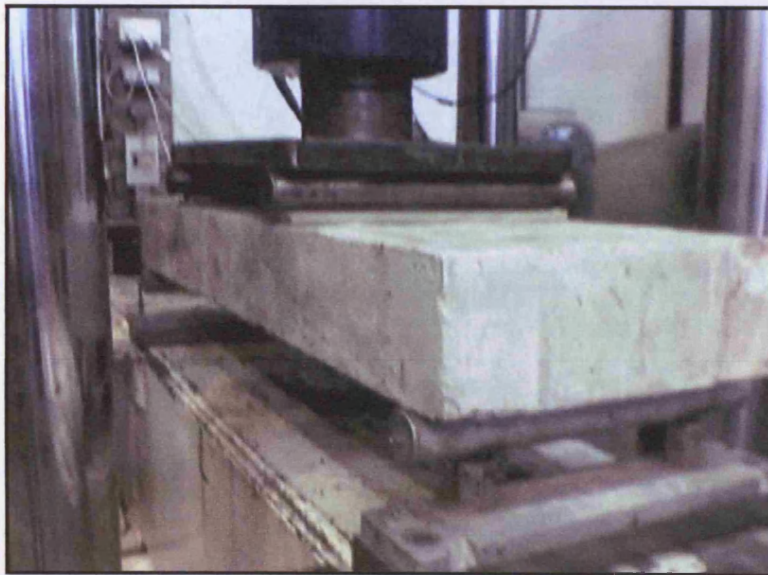
Plate 4.7- Set up for prototype flexural strength test.
