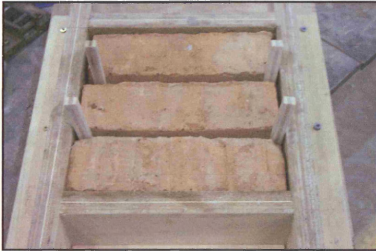
Plate 3.1(a)- Triplet masonry specimen in preparation.
