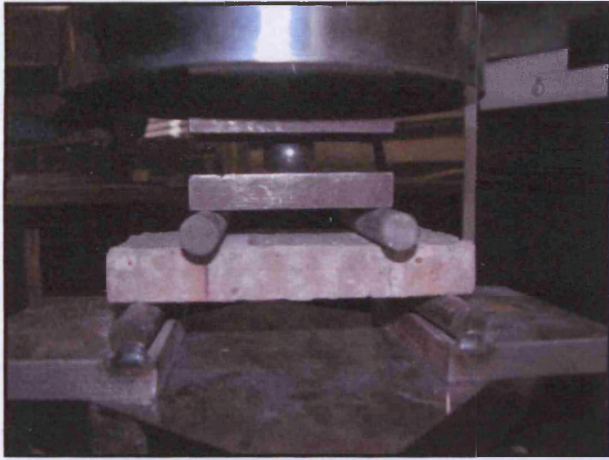
Plate 4.8- Set up for sixth scale flexural strength test.
