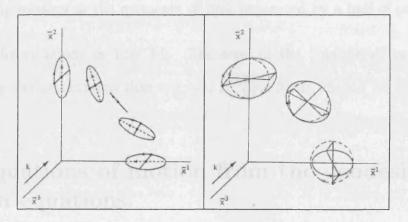
Figure 3.4: Solid lines show 3-dimensional motion of particles, while dashed lines show projections of the trajectories onto the  $\bar{x}^1, \bar{x}^2$  plane. In the left picture the wave is linearly polarized  $(h_+ \neq 0, h_\times = 0)$ , whereas in the right picture the wave is circularly polarized  $(h_+ = h_\times)$ .
