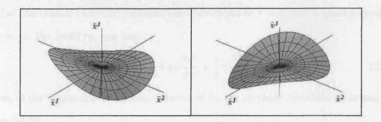
Figure 3.5: The figure shows the deformations of a circular disk of free test particles under the action of a linearly polarized g.w.  $(h_+ \neq 0, h_\times = 0)$ . The "magnetic" contribution is responsible for the displacements along the  $\bar{x}^3$  axis. The two pictures show the configurations at the moments of time separated by a half of period.
