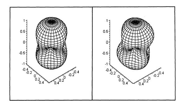
Figure 3.9: The amplitude of the interferometer's response to circularly polarized waves. The graphs are normalized in such a way that the amplitude is equal 1 for  $\Theta = 0$ . The left figure ignores the "magnetic" effect, whereas the right figure shows the total response.
