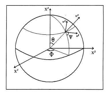
Figure 3.7: The relationship between the coordinate system  $(x^1, x^2, x^3)$  adjusted to the wave and the coordinate system  $(X^1, X^2, X^3)$  adjusted to the interferometer. The two arms of the interferometer lie along the axes  $X^1$  and  $X^2$ .
