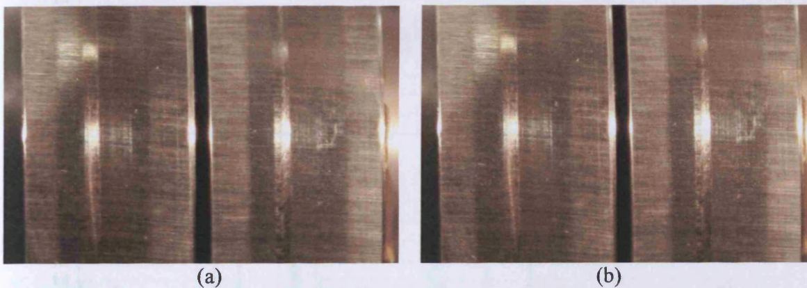
Figure 4.19. Photographs of discs following testing at 16m/s (a) AD09; left: ground disc on fast shaft; right: ground disc on slow shaft (b) AD10; left: ground disc on fast shaft; right: ground disc on slow shaft
