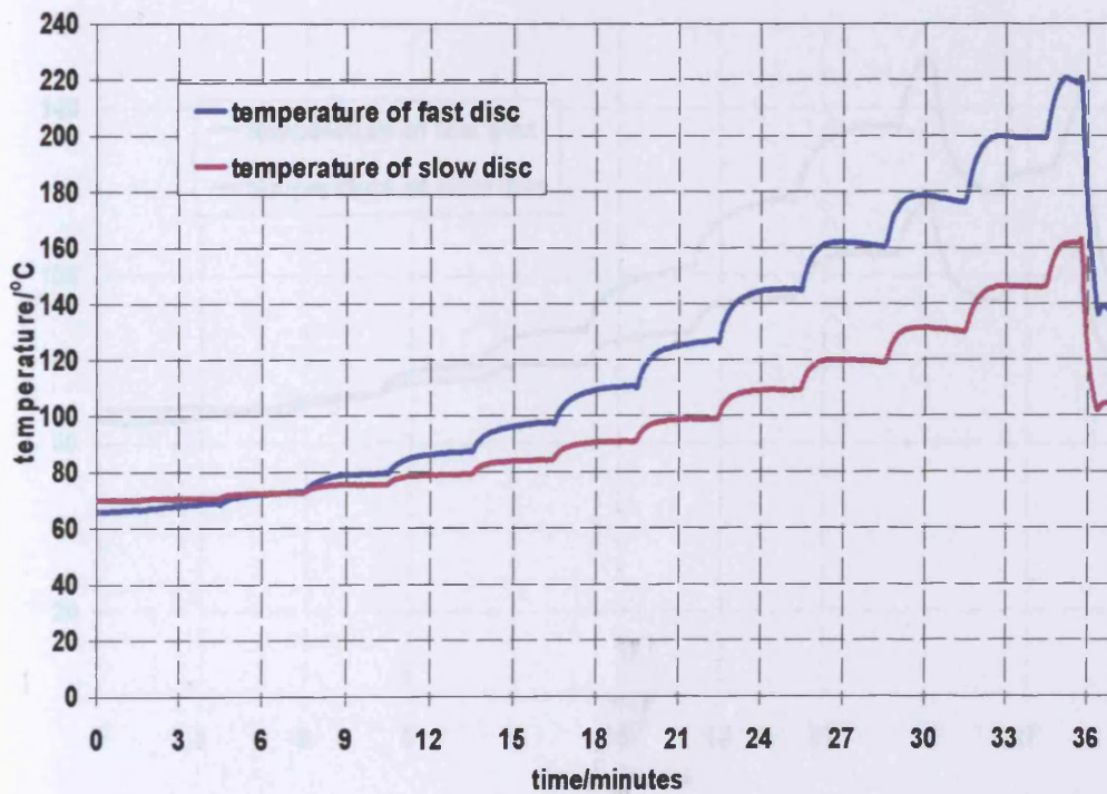
Figure 4.9. Record of scuffing test AD03, upper graph shows applied load and friction force; lower graph shows bulk temperatures of the two discs
