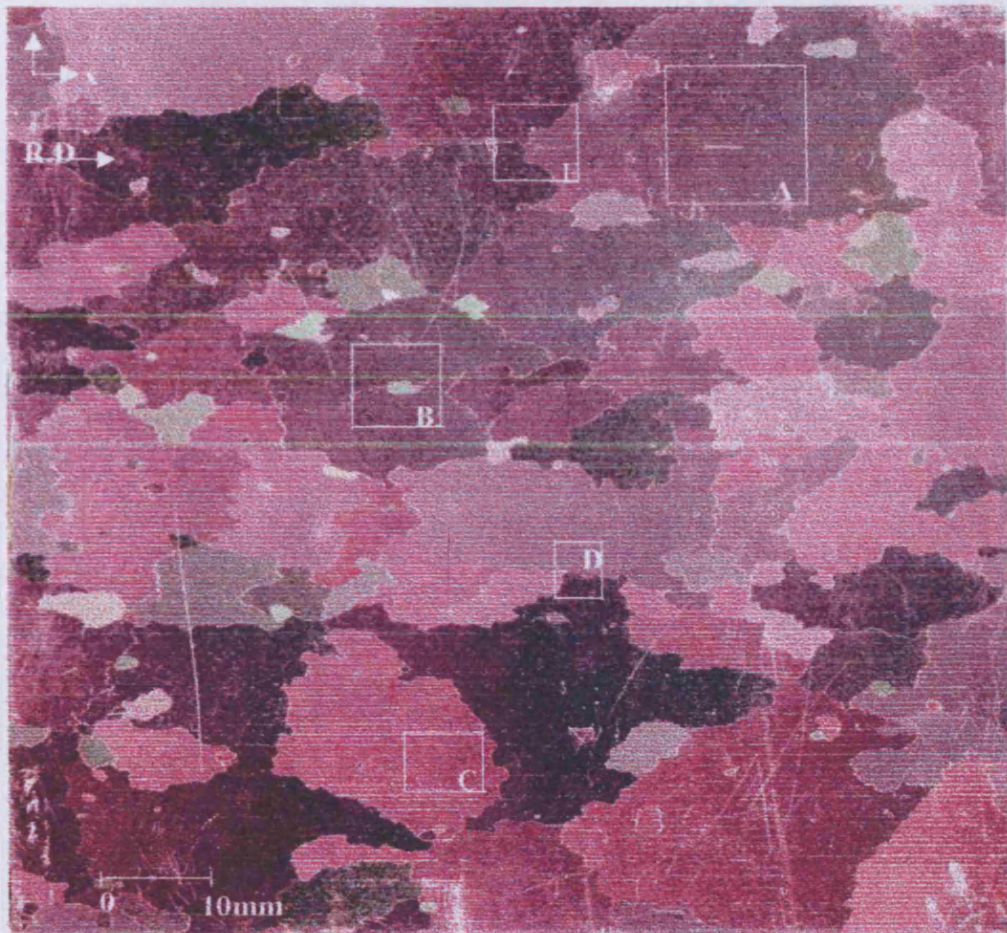
Fig. 8.1: Grain-oriented electrical steel showing regions A, B, C, D and E which were scanned on the top surface.
