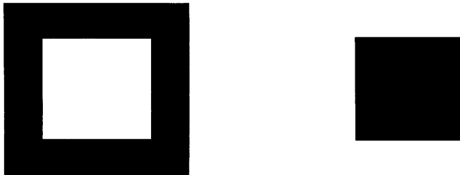
Figure 6-1 Schematic diagram of form of patterns used for edge bead removal, black regions indicate regions of chrome (opaque) and white regions clear glass, the inverse (black = white) of the patterns shown above was also available on the other mask.
