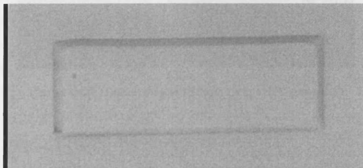
Figure 6-27 Through-microscope picture of the mesa etch with flow baked photoresist on GaN.
