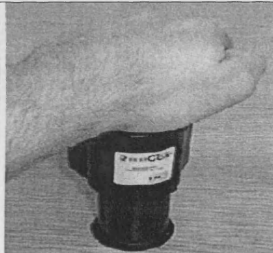
Figure 4.7d : Press Down to Remove Filter Stages.
