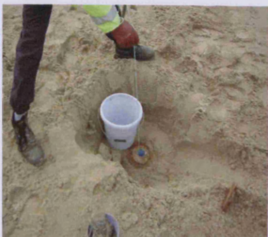
Extracting groundwater from borehole B3 using a bailer (Spring 2005)
