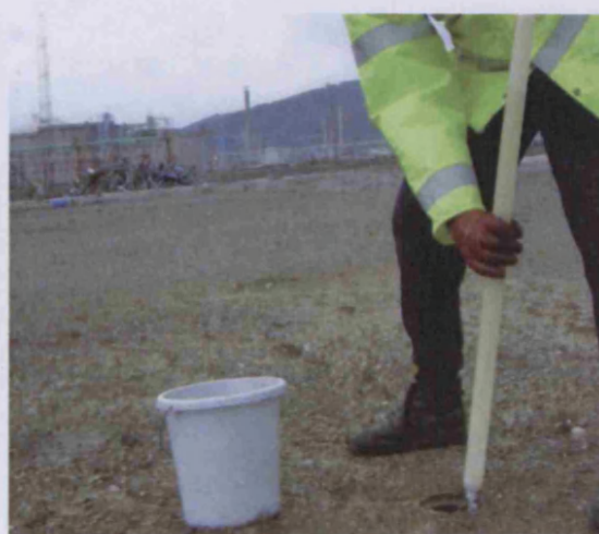
Extracting groundwater from borehole B2 using a bailer (Spring 2005)
