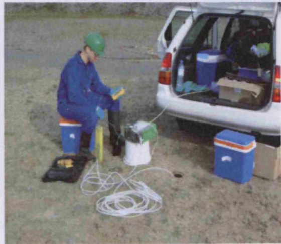
Conducting on site analyses of pH, dissolved oxygen, redox potential and temperature using hand held meters (Spring 2005)
