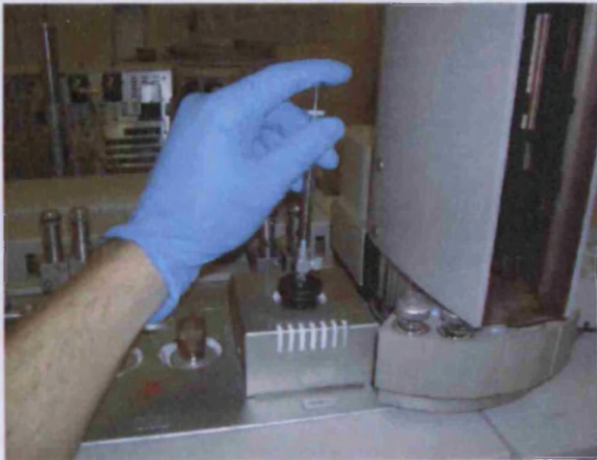
Microcosm headspace samples being directly injected into the GC-MS
