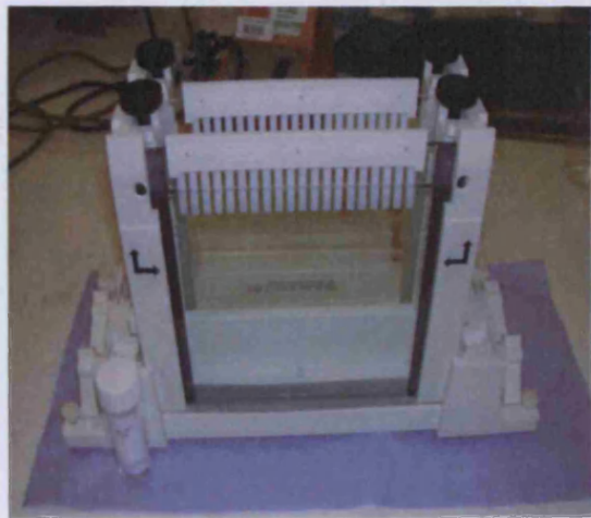
Combs located within the DGGE gels for the formation of injection wells
