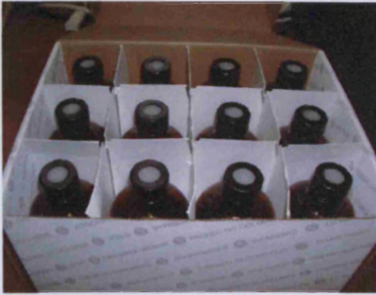
Microcosm bottles sealed with screw on lids and septa
