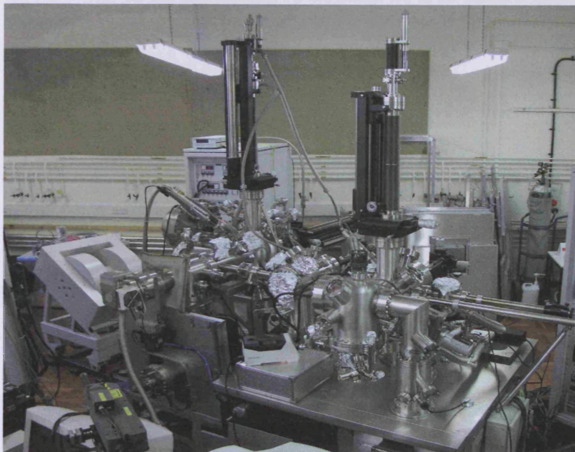
Figure 7.16 The multi-chamber Omicron Multiprobe® Surface Science Ultra-High Vacuum (UHV) system. The EPR magnet is shown in the left of the picture.
