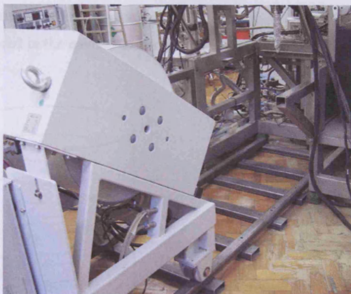
Figure 7.9 The rail system on which the magnet and bridge are situated. The magnet can be rolled into position under the UHV chamber and removed again during bake-out.
