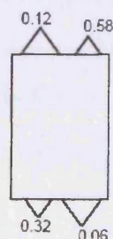
Fig. 2.46: SEM image of the silicon nitride contact tip; each tip holds four cantilevers. On the right the force constant (N/m) is reported next to each cantilever [20].
