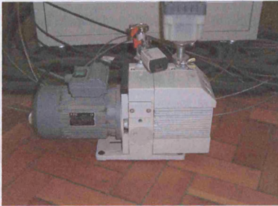
Fig. 2.2: One of the rotary pumps used in the system.
