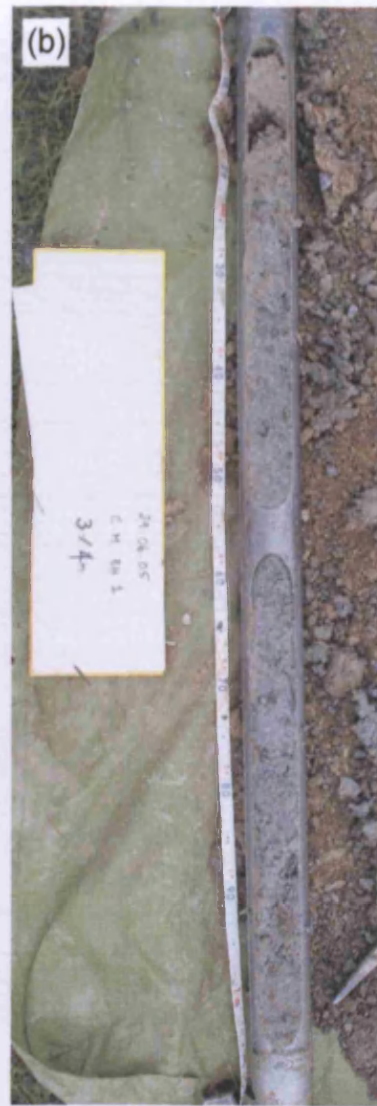
Figure 6.8: Photographs of sediments from Borehole 1 and Borehole 2, Crychell Moor: (a) Sandy fine gravel (diamict), with gravelly silty sand (1.3-1.65 m), 1-2 m, Borehole 1; (b) Silty sandy gravel (diamict), 3-4 m, Borehole 1; (c) Clayey silt, 3-4 m, Borehole 2.
