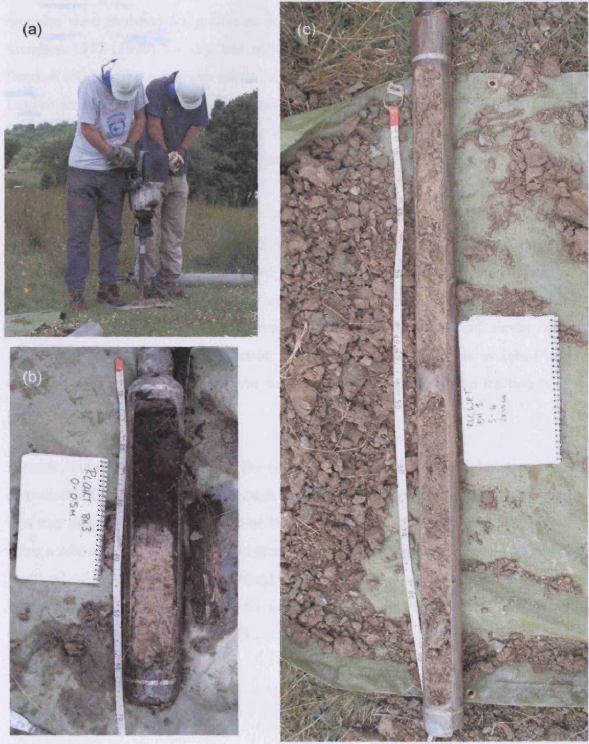
Figure 3.22: Atlas Copco Cobra vibro-coring system used to drill boreholes at sites in Wales. (a) two-stroke percussion drill in operation; (b) 0.5 m long, 95 mm diameter open window core barrel used for the upper 1 m of sediment; (c) 1 m long, 40 mm diameter open window core barrel used for drilling to depth. Photo (a) by P.J. Brabham.
