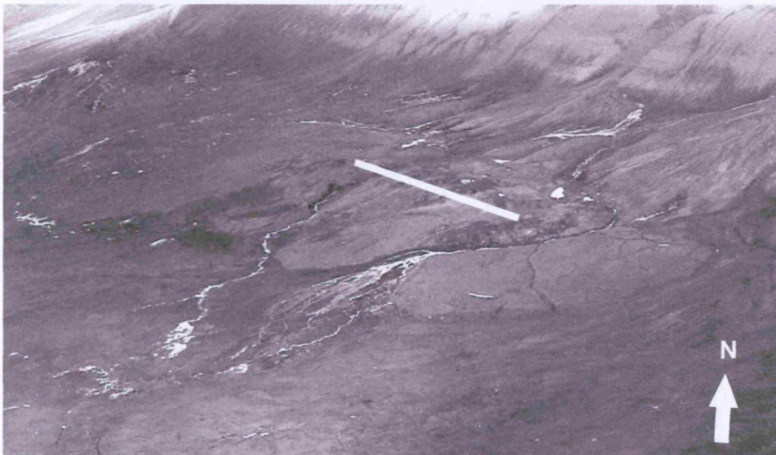
Figure 10.7: Oblique aerial photograph of Hytte pingo. The location of the electrical resistivity survey line is indicated.
