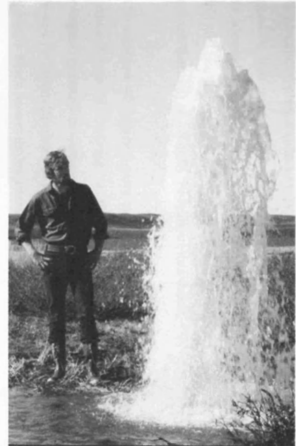
Figure 2.3: Drill-hole flow from the sub-pingo water lens of a closed system pingo ('Pingo 14'), 20 km east of Tuktoyaktuk, N.W.T., Canada (from Mackay 1998) (Photo: J.R. Mackay).
