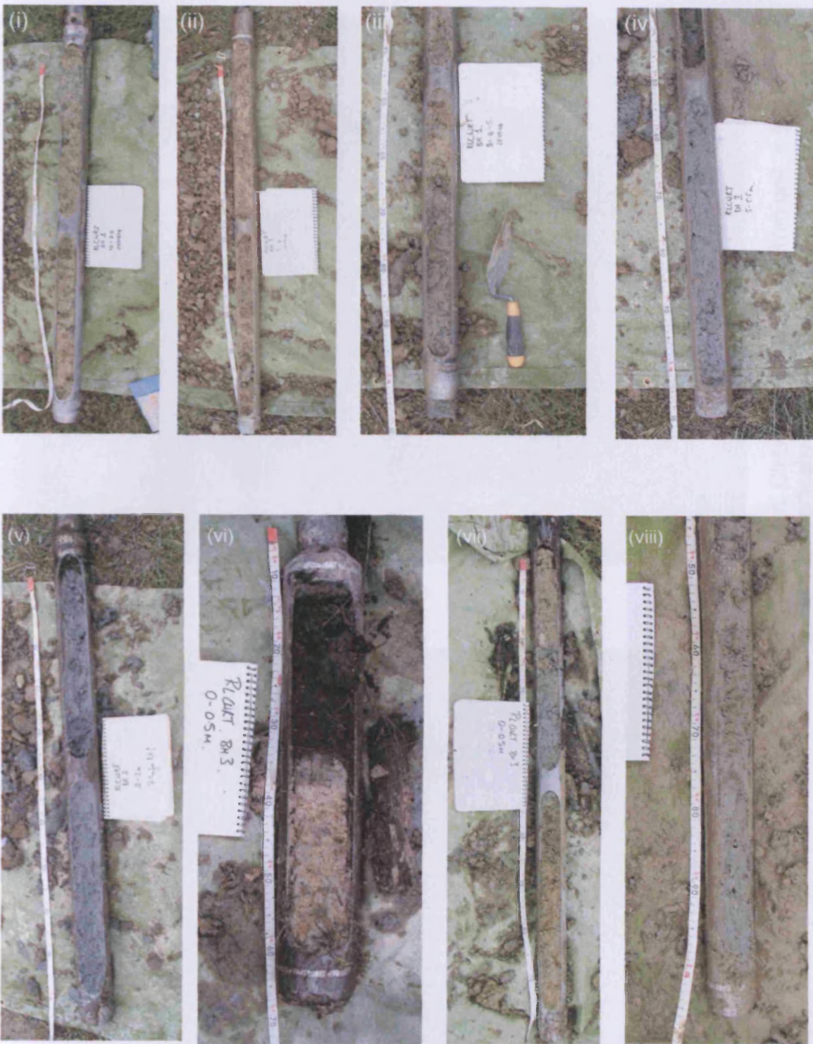
Figure 8.9a: Photographs of borehole cores from 'Pingo' 3, Rhos Llawr Cwrt, Cletwr valley. Borehole 1: (i) gravelly, slightly sandy, clayey silt (1-2 m) (Photo: C. Harris); (ii) clayey silty gravel (3-4 m); (iii) silty fine gravel underlain by clayey silt (4.5-5 m); (iv) clayey silt with occasional clasts (5-5.5 m). Borehole 2: (v) sandy, silty clayey gravel (2-3 m). Borehole 3: (vi) peaty organic topsoil underlain by weathered sandy, clayey silt (0-0.5 m); (vii) silty sandy gravel (1-2 m) (Photo: C. Harris); (viii) finely laminated clayey silt (4.5-5 m) (Photo: C. Harris).
