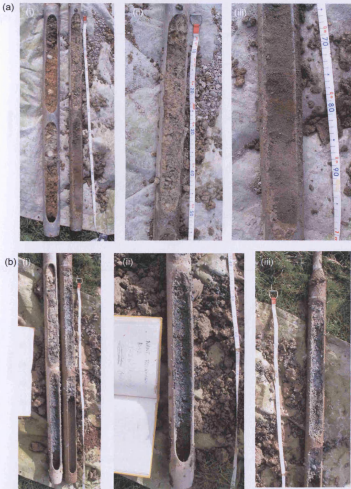
Figure 5.8: Core photographs, Llanio Fawr: (a) Borehole NB1: (i) poorly sorted sandy gravels and diamict units (1-2 m) (left hand core) grading downwards to well sorted fine sand (2-2.9 m) (right hand core); (ii) poorly sorted sandy gravel (2-2.5m); (iii) well-sorted sand and sandy silt (2.7-3 m); (b) Borehole NB2: (i) poorly sorted sandy gravel/diamict (1-2 m) (left hand core) grading downwards into a gravelly sand (2-2.6 m) (right hand core); (ii) well sorted gravelly sand (1.5-2 m); (iii) well sorted gravelly sand (2-2.6 m).
