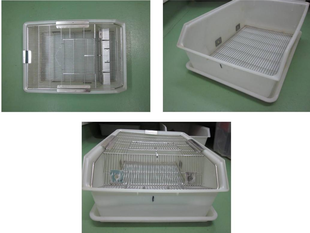
**Figure 2.2.2:** Images of the activity chambers: a) view from above; b) a view from the side; c) front view of the chambers.
