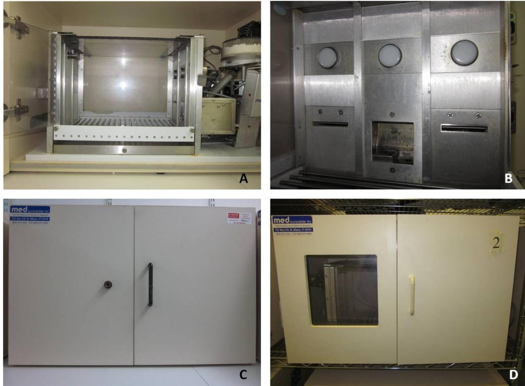
**Figure 2.2.1:** Images of the operant chambers: a) view inside the operant box; b) view of recess magazine (lever slots are visible on either side of the magazine); c) front view of the chambers housing the boxes in set A; d) front view of the chambers housing the boxes in set B.
