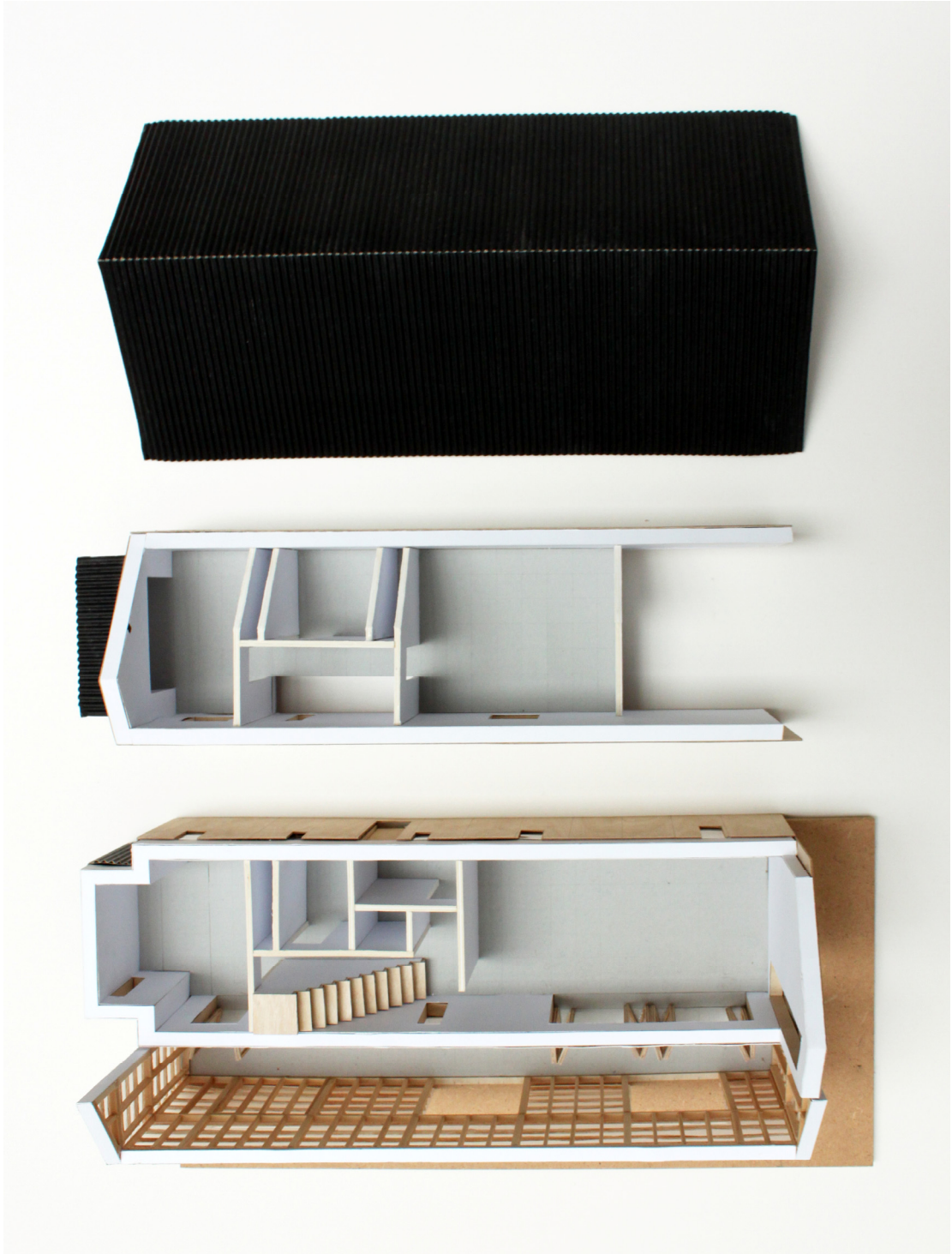
Fig. 4.80 Model showing the construction and material finishes, in addition to the spatial layout and setting out of standard sized materials
