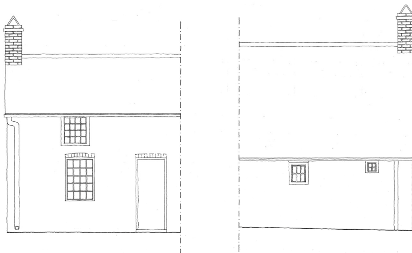
Fig. 6.11 Simple south-west and north-east elevations at Rhydycar also display environmental and functional influences 1:100
