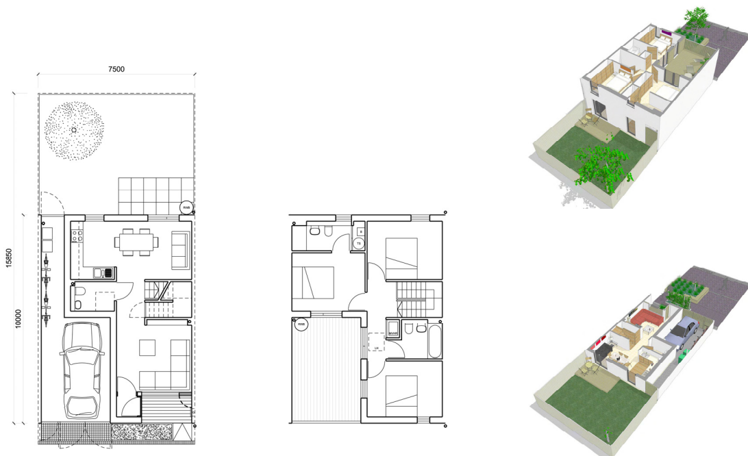
Fig. 6.28 Ground and first floor plans of the 3 bed house type; Fig. 6.29 Spatial study of 3 bed house type
