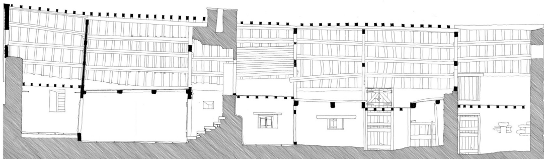
Fig. 8.5 Measured drawing of Llannerch y cawr showing form and construction, devoid of signs of inhabitation
