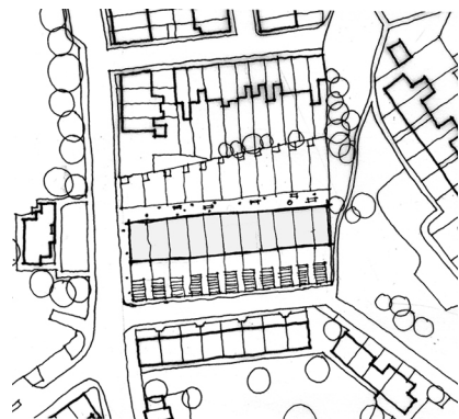
11 houses Small back gardens and large front garden allotments, long plots with N/E orientation with parking at the rear
