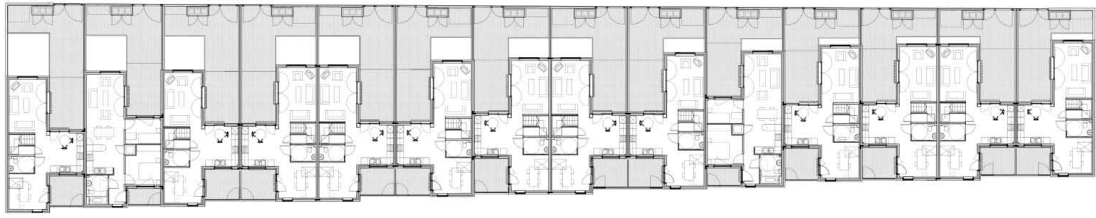
Fig. 6.36 T-shaped house plans arranged in different ways to form the street
