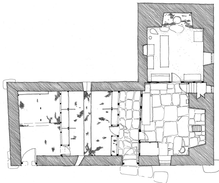
Fig. 4.24 Plan of Cilewent showing the cow house to the left and the living quarters to the right. It also demonstrates the different material finishes of the floor relating to the functions of the house 1:200
