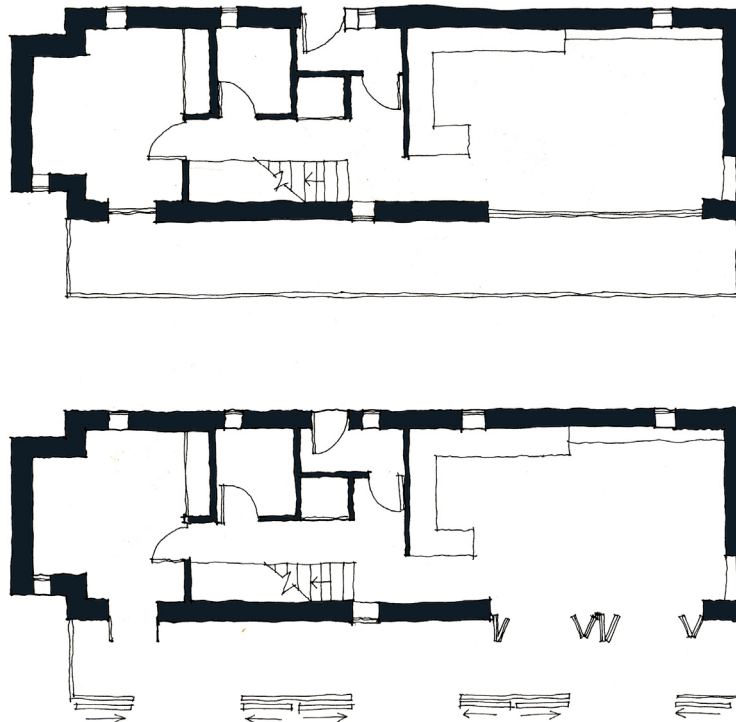
Fig. 4.73 South façade closed up in cold weather in winter and opened in warm weather in summer
