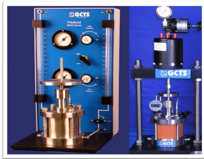
Figure 2.6. A photograph showing Fredlund SWCC device (GCTS Testing Systems).
