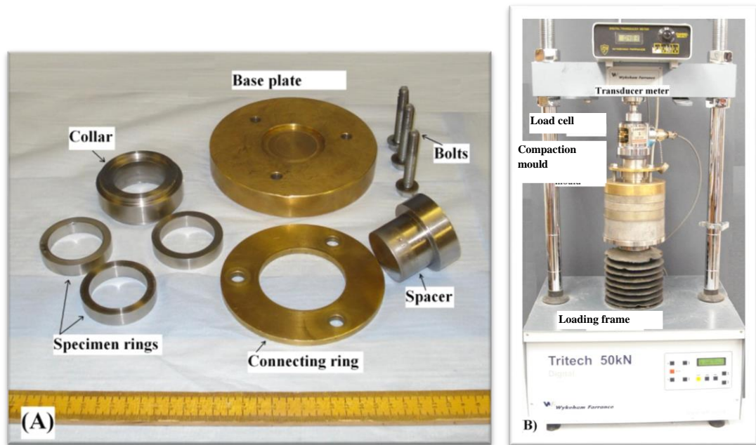
Figure 3.4. Photographs showing (a) compaction mould components, (b) compaction setup for specimens used for SWCC tests.
