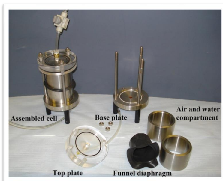
Figure 4.9. A photograph of disassembled and assembled manometer cell.
