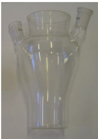
Figure 1.12: A simple undivided cell for electrolysis
