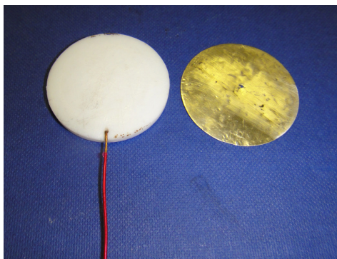
Figure 2.11: The PTFE constructed electrodes
