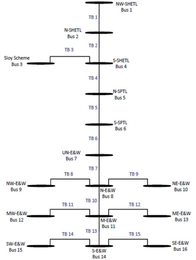
Fig. 4. GB 16 busbars electricity network. The load locates at all the busbars except Bus8 and Bus11.
