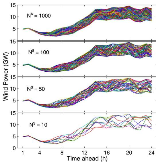
Fig. 9. Different number of wind power forecast scenarios derived by applying the scenario reduction algorithm on 1000 randomly generated scenarios.  $N^s$  is the number of wind power forecast scenarios.
