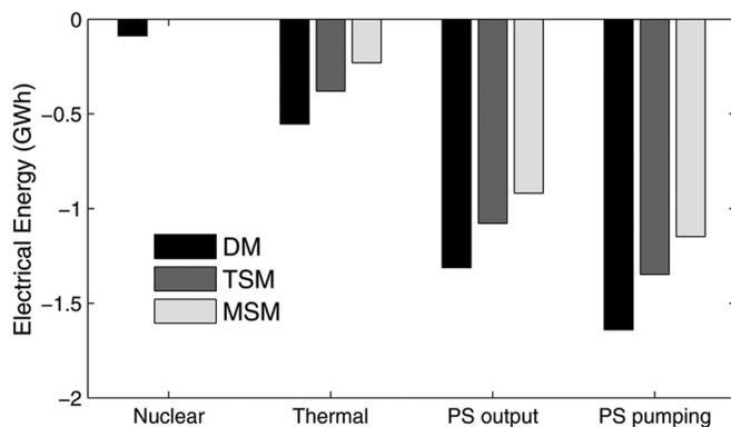
Fig. 14. Changes in expected electrical energy production from different types of generation units in various methods with respect to the energy production in PFM.
