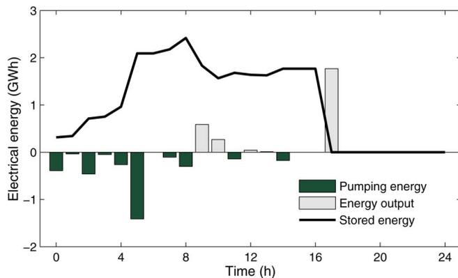
Fig. 15. Total electrical energy used for water pumping, and electrical energy produced by pumped storage units in the PFM.
