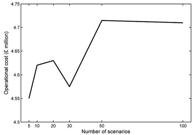
Fig. 11. Comparison between operational cost of the electricity network for different number of forecast scenarios. This comparison was done to test the stability of a scenario reduction algorithm.
