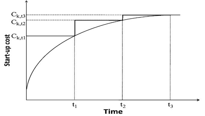
Fig. 2. Discretized startup cost for thermal generating units. The horizontal axes shows time length in which a thermal generating unit remained OFF, before starting up.
