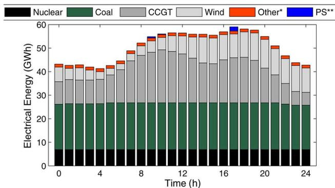
Fig. 13. Power output from different types of generator for the perfect foresight method. \* Including Biomass, CHP, and Hydro. \*\* Pumped Storage.
