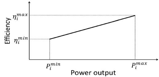
Fig. 3. Linear approximation of part-load efficiency for thermal generating units.
