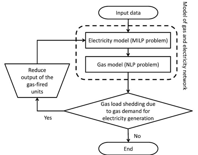
Fig. 1. Structure of the integrated gas and electricity network model.
