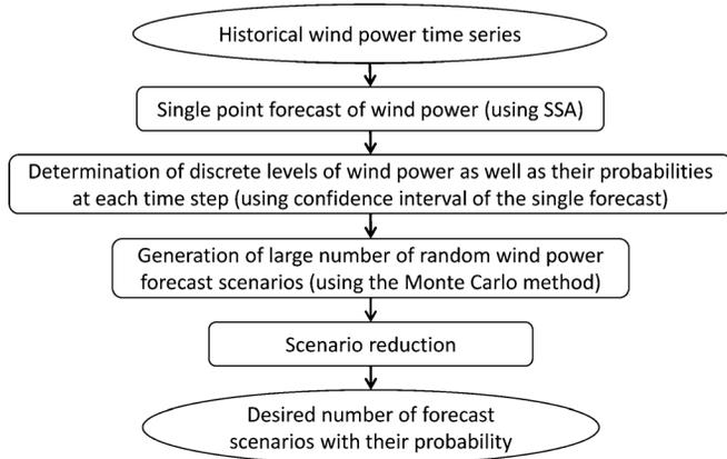
Fig. 8. Algorithm for producing probabilistic wind power forecasts.
