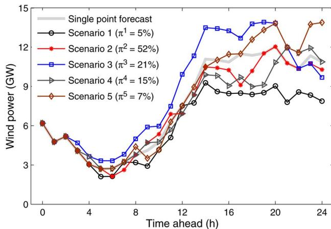
Fig. 10. Probabilistic wind power forecast scenarios and the single point forecast.  $\pi^s$  represents the probability of the  $s$ th forecast scenario.
