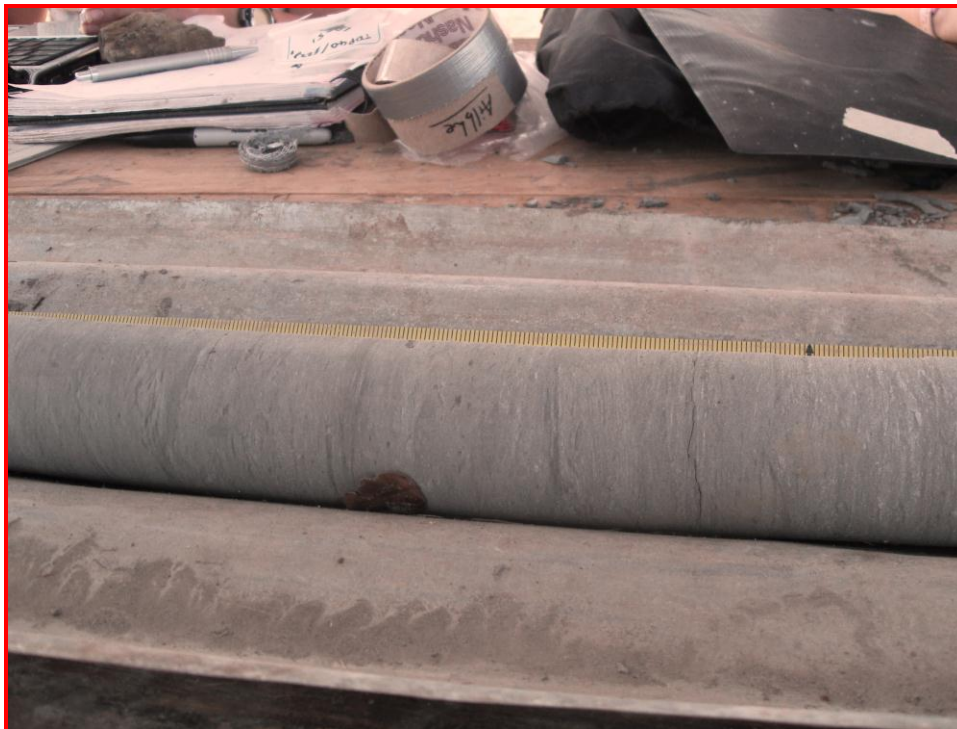
Fig. 2.2h: A core has been placed in a working bench for describing and sampling after being photographed.
