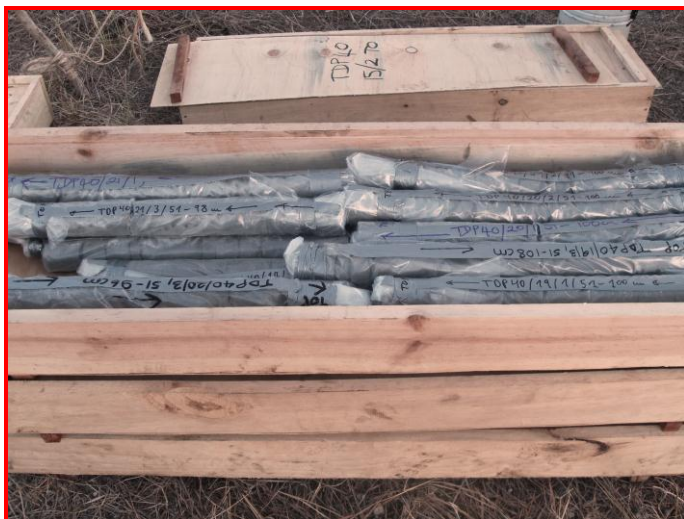
Figure 2.2i: Showing Cores are properly packed and ready for transport to Dar es Salaam. After sampling the remaining core material is wrapped in plastic and placed in wooden core boxes for storage and future use.
