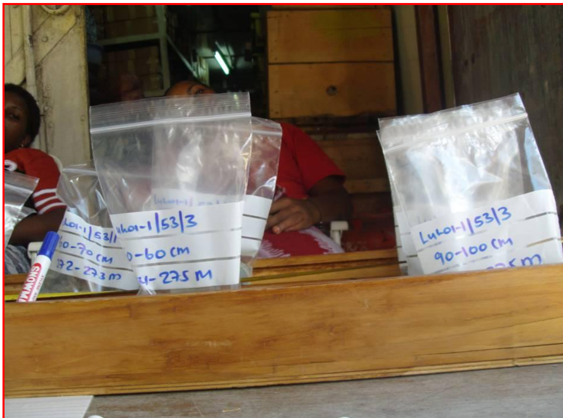
Figure 2.4: Photograph showing examples of labeled core samples; plastic bags showing well named core section, interval taken in cm and depth in the borehole in metres.
