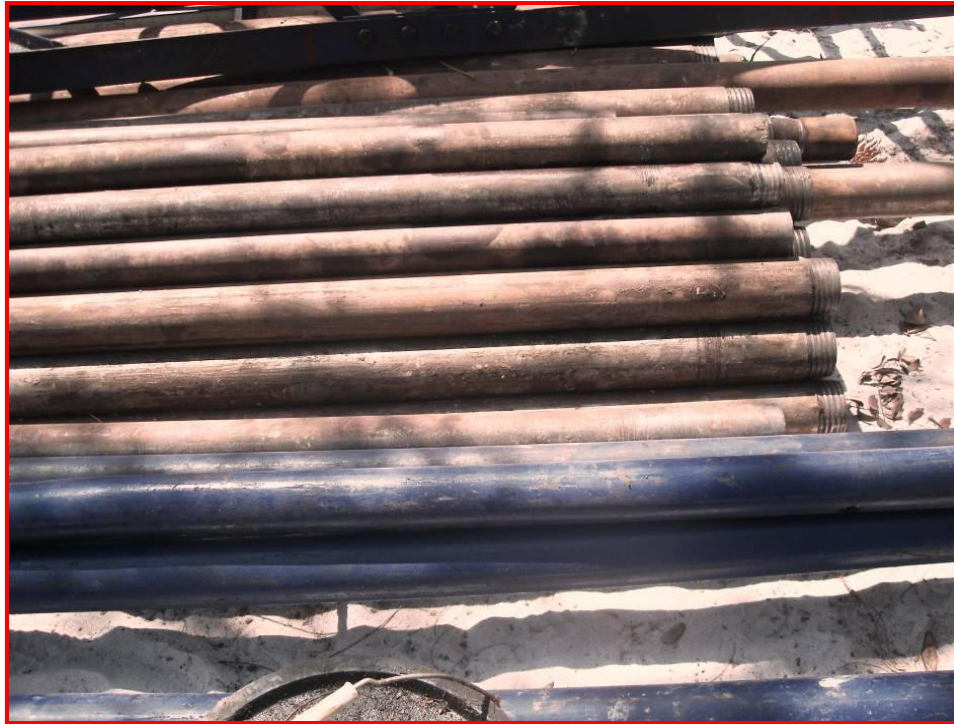
Figure 2.2e: Photograph showing drilling rods used for drilling TDP Site 40 Holes A and B.
