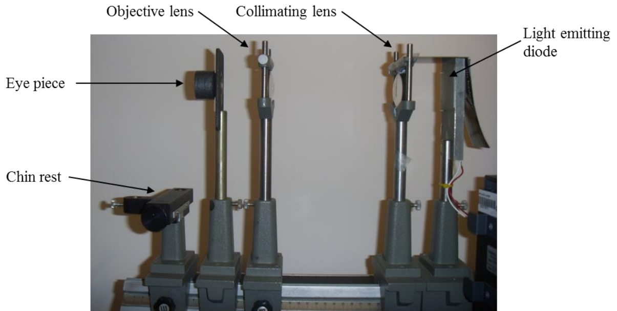
Figure 4.3 Photograph showing the Maxwellian View optical system used to administer an equilibrium bleach.
