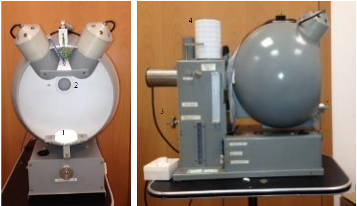
Figure 3.8 The Goldmann-Weekers adaptometer. 1 = patient chin rest; 2 = light stimulus; 3 = examiner controls to adjust stimulus illumination; 4 = rotating drum and logarithmic paper.
