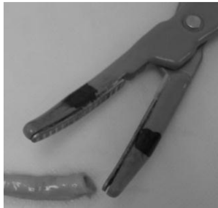
Figure 3-9 Image showing sealing region marked on the device to eliminate the variation in application force due to positioning of the vessel within the jaws of the device.
