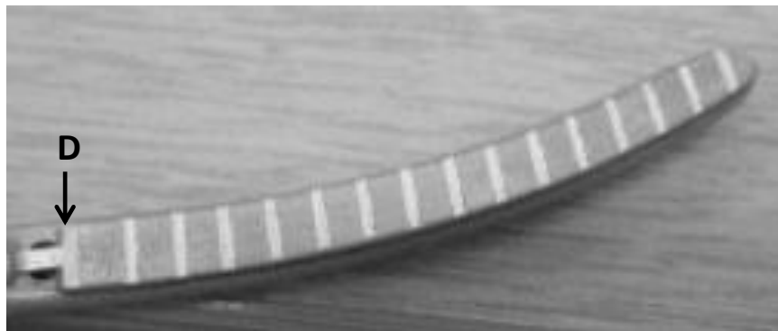
Figure 3-8 Image showing a modified shim of the PlasmaKinetic OpenSeal device, with the straight edge used as a datum for producing the grooves indicated by D .
