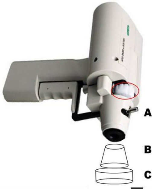
Figure 2.3 Diagram of modified Helios® gene gun. Diagram showing approximate, relative position at the time of use. A – Helio® gene gun with barrel removed to allow for closer proximity to the filter. The red circle shows the barrel containing the Dil/DiO loaded tubing. B – Falcon-filter in position to scatter the fired tungsten particles. This was designed to create a more uniform spread of particles and filter out larger particles to reduce kinetic damage to the tissue. C – Cell culture insert with retina to be labelled mounted on the upper surface. Scale bar = 1cm.
