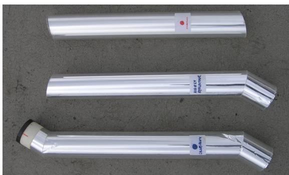
Figure 8 The three tested sky-tube types. From the top: A (no bends), B (one bend), C (two bends).
