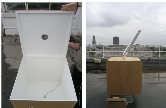
Figure 7 The scale model installation - (left) inside the box and (right) box with sky-tube.
