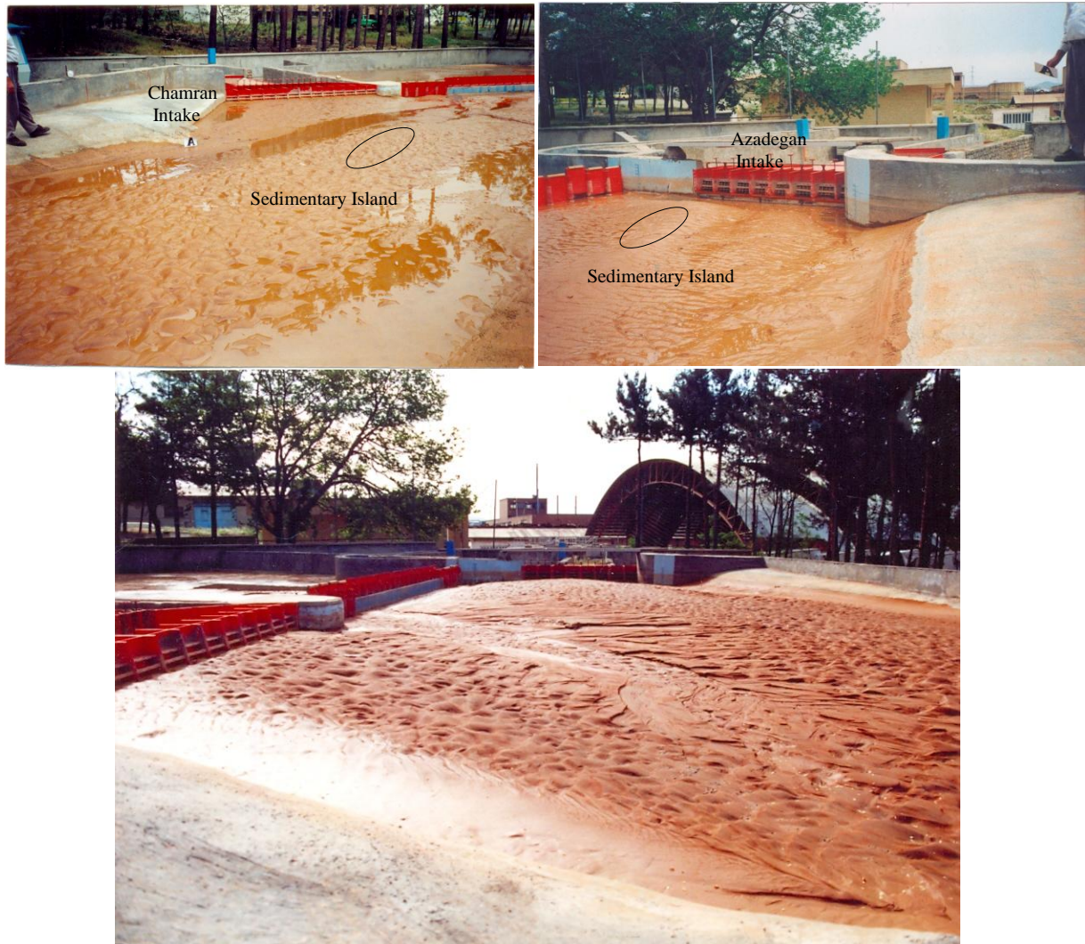
Figure 3.31 Morphological changes in Hamidieh regulated reservoir (physical model) after sediment transport experiments
