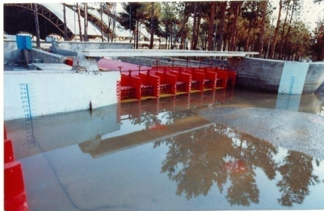
Figure 3.13 Putting gage marks in the physical model
