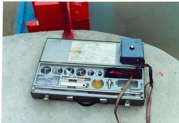
Figure 3.14 Mechanical current meter system (A.OTT KEMPTEN, type: C 2 . "10.150", NO.52051-meter support on rod of 9 mm diameter)
