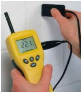
Figure 3.1 – Picture of Protimeter MMS
