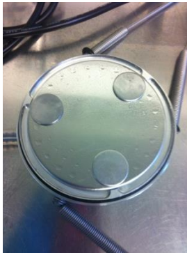
Figure 4.2 – Position of three stainless steel discs within cascade impactor
