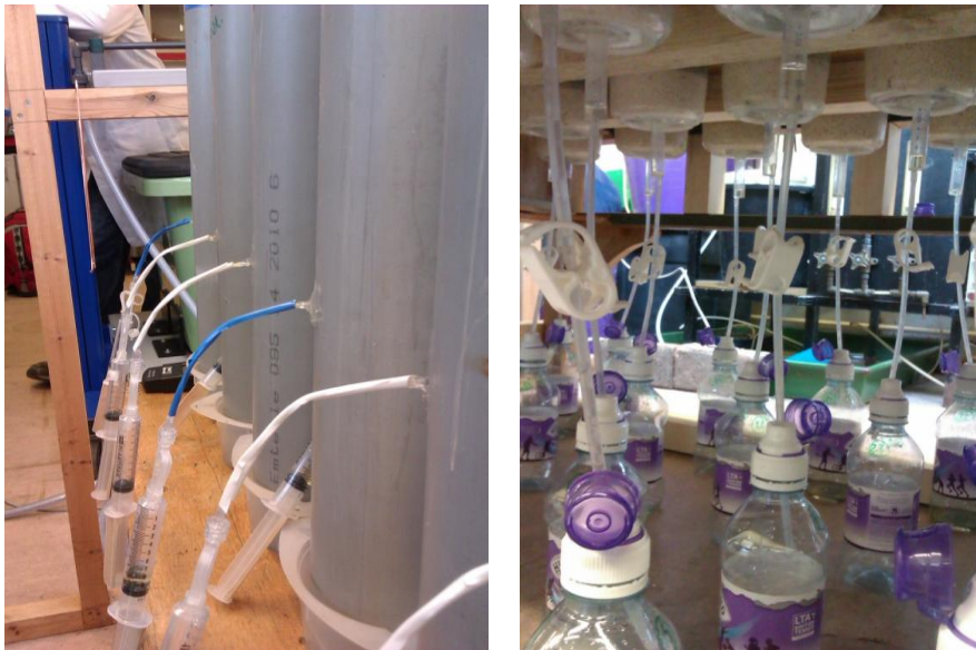
Figure 3.11 Column Growth trials set up with Rhizon and base sampling points.
