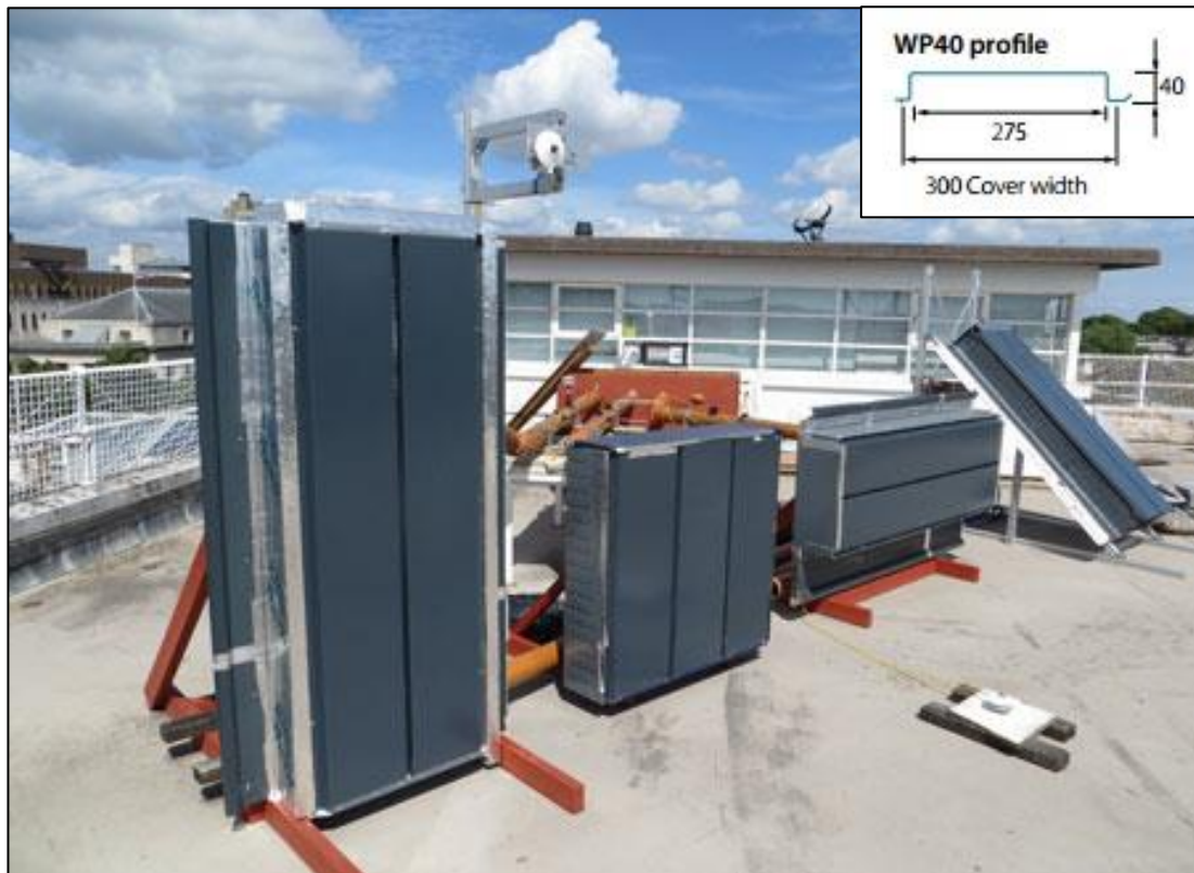
Figure 5-63: TSC prototype assembled, the profile used is shown in the top-right corner (photo was taken by SBED team)
