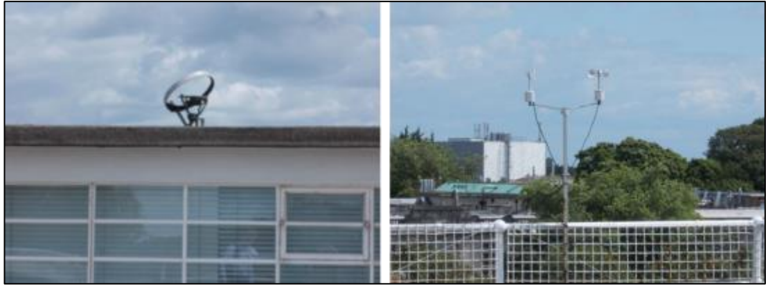
Figure D-7: (a) Existing solar irradiation diffuser (b) Existing weather station – remedial work is required for the relative humidity and temperature sensors
