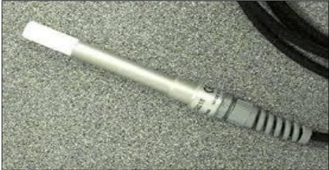
Figure D-13: (a) CS215-L Temperature and Relative Humidity Sensor, (b) HMP155A-L Temperature and Humidity Probe
