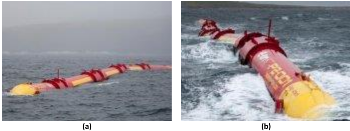
Figure 6 Pelamis operating in Orkney (Pelamis Wave Power Ltd., 2013a) (a) in 2011 (b) in 2012 .
