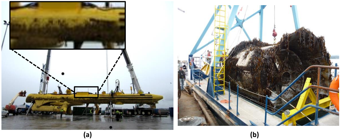
Figure 39 Biofouling on the (a) SR250 turbine (Scotrenewables, 2013) (b) Clean Current turbine (Clean Current, 2007)
