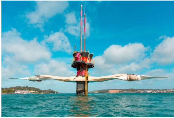
Figure 11 SeaGen - example of a tidal stream turbine (Marine Current Turbines Ltd., 2013a)
