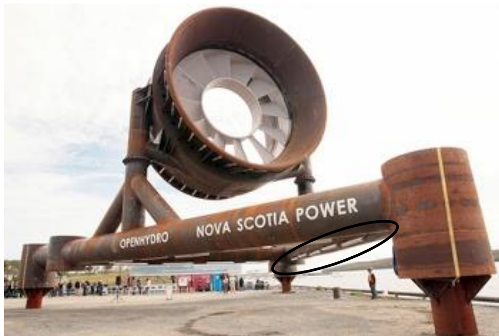
Figure 37 OpenHydro support structure with sacrificial anodes (circled) (Snohomish County Public Utility District, 2012)
