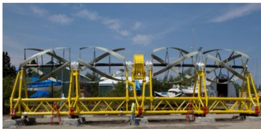
Figure 21 TidGen, an example of a THATT (Maine Technology Institute, 2013)
